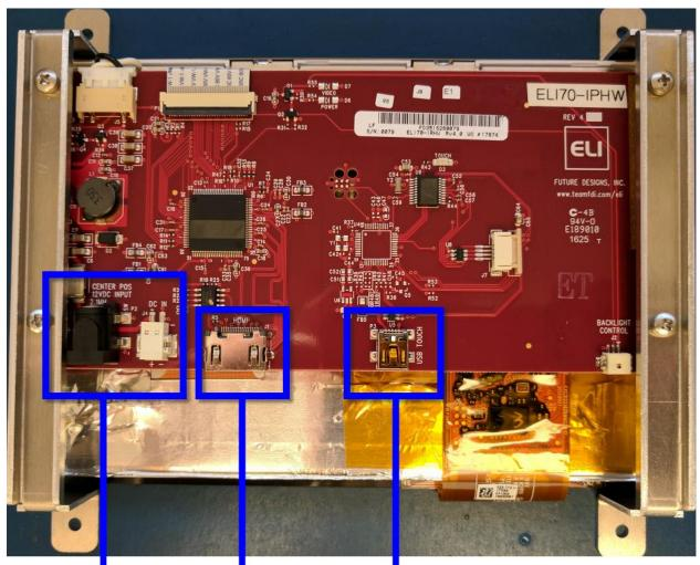
Power HDMI USB Mini-B Input Input Touch
