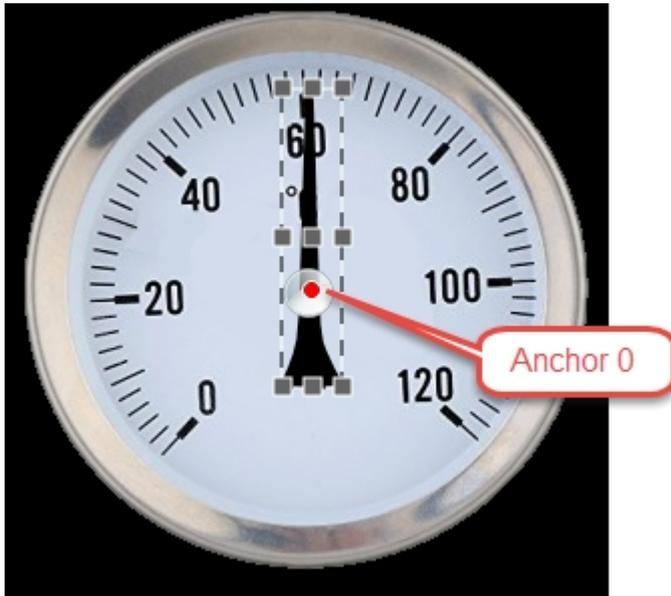
Example: The pointer should rotate around the centre of the circle. The pointers 9 standard anchors (shown in dark grey) are not useful in this case because none of the defaults are located in the right position. The anchor 0 can be placed pixel-precise ([#OAS](#)) as shown, and this custom location marks the correct rotation point for the pointer object.
