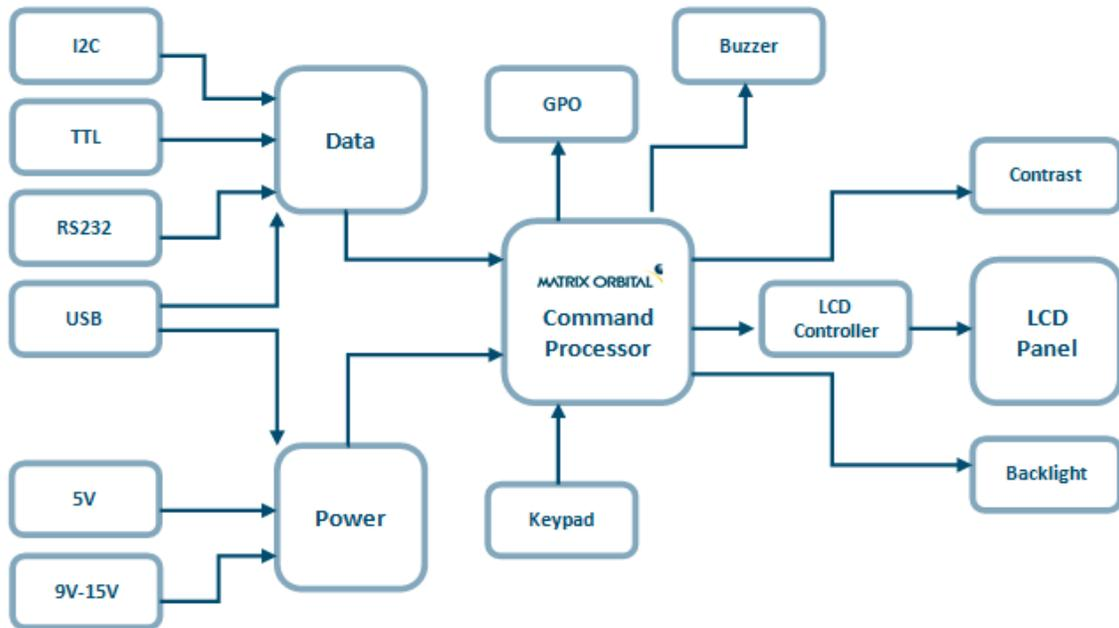
Figure 15: Functional Diagram
