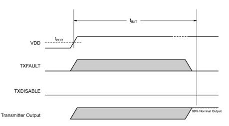
Figure 15. Initialization Timing with TXDISABLE Asserted
