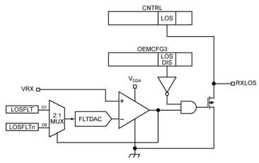
Figure 12. RXLOS Comparator Logic
