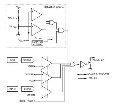
Figure 10. Fault Comparator Logic
