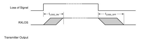
Figure 17. Loss-of-Signal (LOS) Timing
