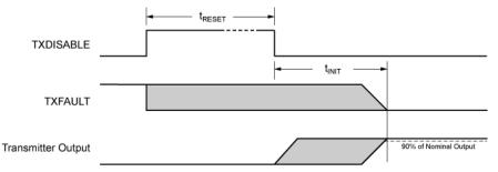
Figure 19. Successfully Clearing a Fault Condition
