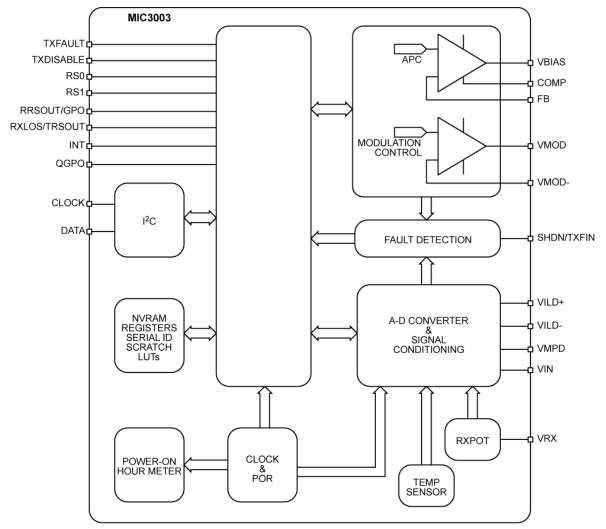
Figure 1. MIC3003 Block Diagram
