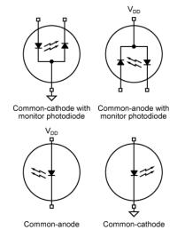
Figure 7. Transmitter Configurations Supported by MIC3003
