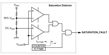
Figure 11. Saturation Detector
