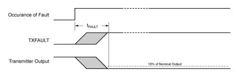
Figure 18. Transmit Fault Timing
