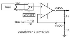
Figure 8. V<sub>MOD</sub> Configured as Voltage Output with Gain
