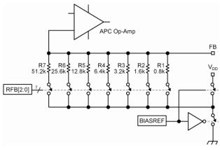
Figure 6. Programmable Feedback Resistor
