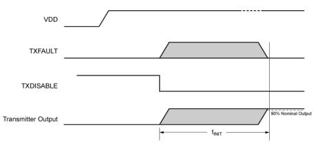
Figure 16. Initialization Timing with TXDISABLE Not Asserted
