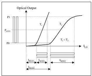
Figure 1. Laser behavior changes over temperature
