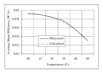
Figure 3. Laser average slope efficiency change over temperature ( $P_{AVG} = -4dBm$ ): from measurement and from calculation
