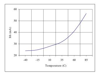
Figure 2. Laser threshold change over temperature
