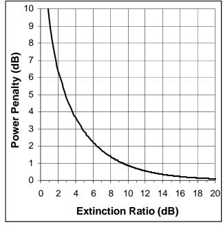
Figure 4. Power penalty vs. extinction ratio (dB ratios)
