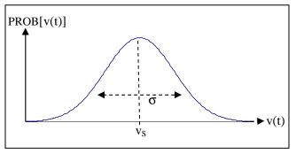
Figure 1. AWGN probability density function
