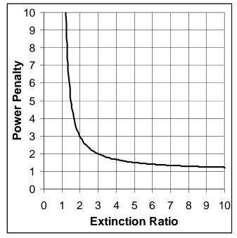
Figure 3. Power penalty vs. extinction ratio (linear ratios)
