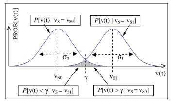
Figure 2. Probability of error for binary signaling
