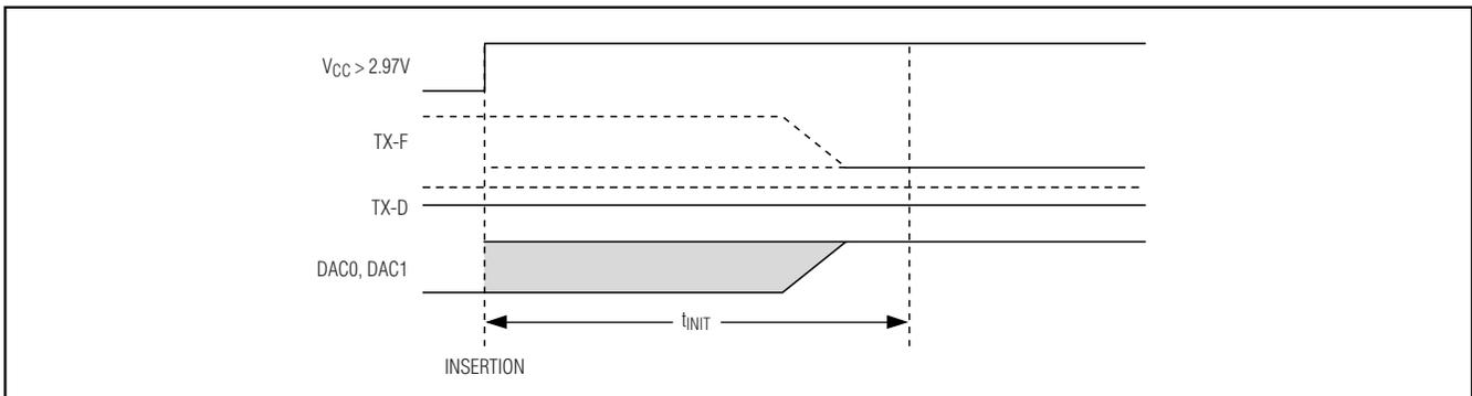
Figure 3. Example of Initialization with TX-D Low (Hot-Plug)
