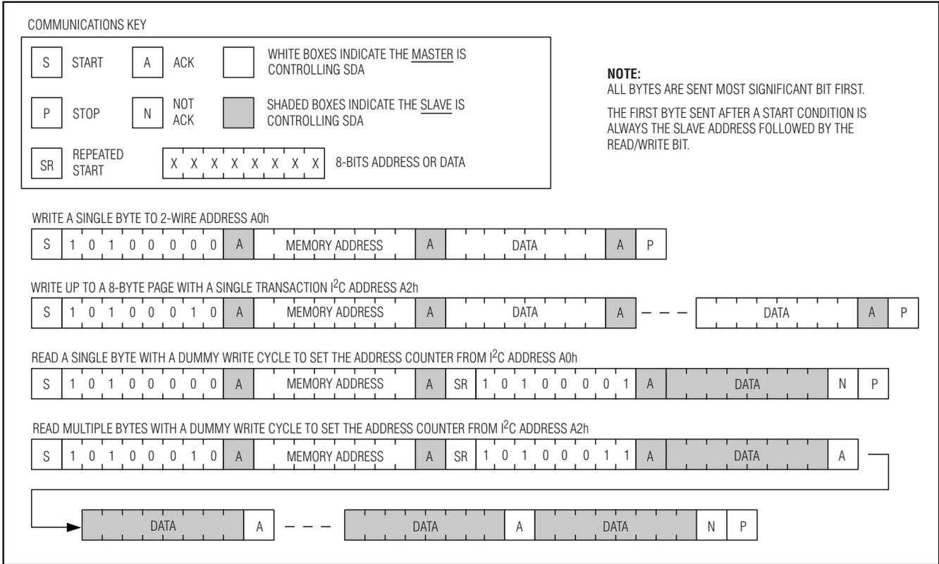
Figure 20. I<sup>2</sup>C Communications Examples
