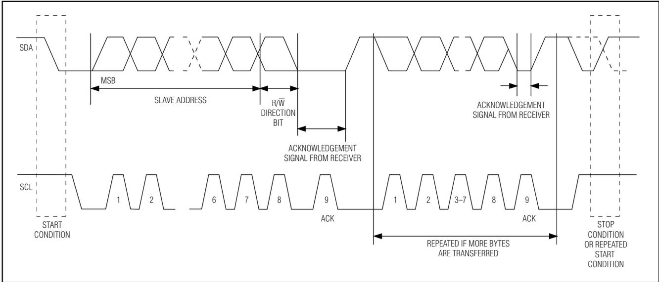
Figure 18. I<sup>2</sup>C Data Transfer Protocol
