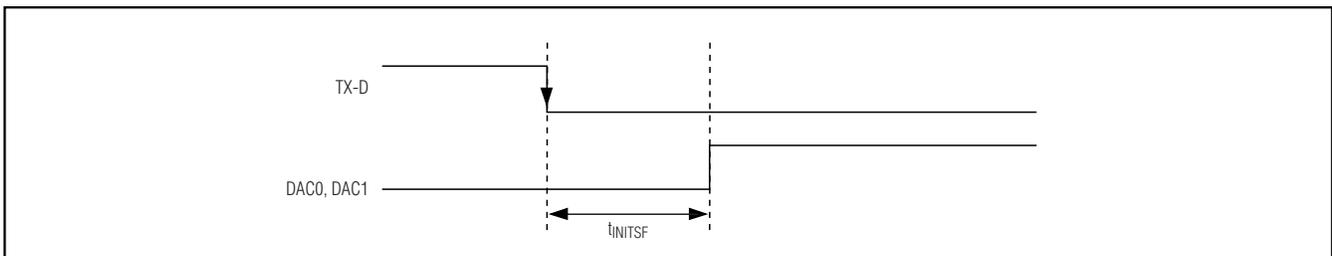
Figure 10. Output Enable/Recovery from Safety Fault Shutdown
