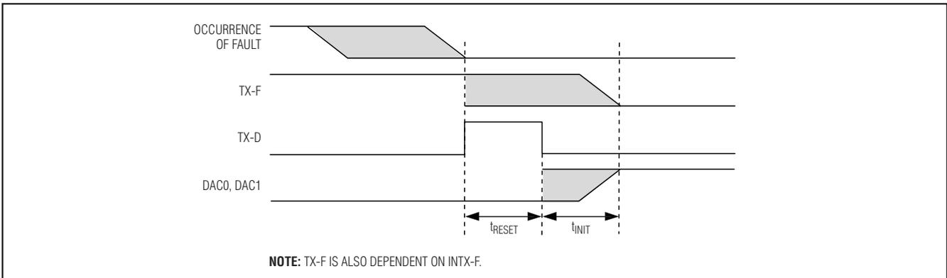
Figure 6. Successful Recovery from Transient Safety Fault Condition
