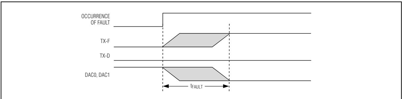
Figure 5. Detection of Transmitter Safety Fault Operation
