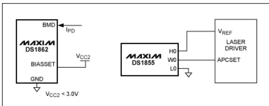
Figure 3. BIASSET current-to-voltage conversion circuit.
