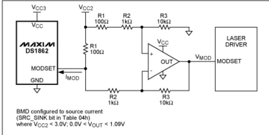
Figure 2. MODSET current-to-voltage conversion circuit.
