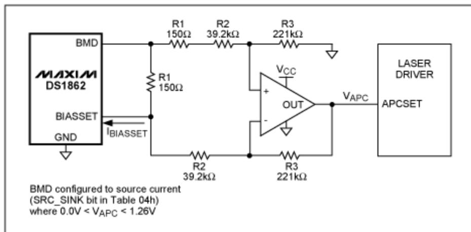
Figure 1. BIASSET current-to-voltage conversion circuit.
