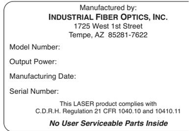
**Figure 3. Laser certification and identification label.**
