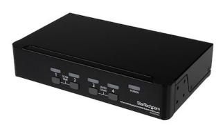
The SV431DPUA 4 Port USB DisplayPort KVM Switch with Audio combines next generation display standards with seamless KVM control of up to 4 connected PC or Mac computers.
