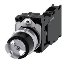
RONIS key-operated switch, 22 mm, round, metal, shiny, lock number SB30, with 2 keys, 2 switch positions O-I, latching, actuating angle 90°, 10:30h/13:30h, key removal O+I, with holder, 1 NO+1 NC, spring-type terminal, possible special locks: SB31, 421, 455 upper case and lower case, always upper case at the beginning of the word
