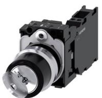
RONIS key-operated switch, 22 mm, round, metal, shiny, lock number SB30, with 2 keys, 2 switch positions O-I, latching, actuating angle 90°, 10:30h/13:30h, key removal O+I, with holder, 1 NO+1 NC, spring-type terminal, possible special locks: SB31, 421, 455, upper case and lower case, always upper case at beginning of line
