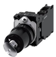
key-operated switch Siemens, 22 mm, round, plastic, lock number SSG10, with 2 keys, 2 switch positions O-I, latching, 10:30h/13:30h, key removal O+I, with holder, 1 NO+1 NC, spring-loaded terminal, with laser labeling, lower case
