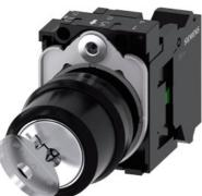
RONIS key-operated switch, 22 mm, round, plastic, lock number SB30, with 2 keys, 2 switch positions O-I, latching, 10:30h/13:30h, key removal O+I, with holder, 1 NO, spring-type terminal, possible special locks: SB31, 421, 455, with laser labeling, upper case and lower case, always upper case at beginning of line
