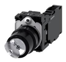
RONIS key-operated switch, 22 mm, round, plastic, lock number SB30, with 2 keys, 2 switch positions O-I, latching, 10:30h/13:30h, key removal O+I, with holder, 1 NO+1 NC, screw terminal, possible special locks: SB31, 421, 455, with laser labeling, upper case and lower case, always upper case at the beginning of the word
