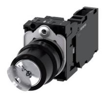
RONIS key-operated switch, 22 mm, round, plastic, lock number SB30, with 2 keys, 2 switch positions O-I, latching, 10:30h/13:30h, key removal O+I, with holder, 1 NO+1 NC, screw terminal, possible special locks: SB31, 421, 455
