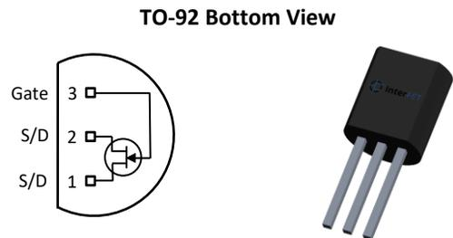
NOTE: S/D pins are interchangeable Source Drain connections
