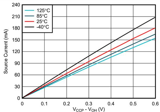
Figure 5-18. I/O Source Current vs Output High Voltage, V<sub>CCP</sub> = 3.6 V
