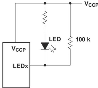
**Figure 8-2. High-Value Resistor in Parallel with LED**
