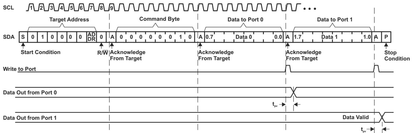
**Figure 7-9. Write to Output Port Register**
