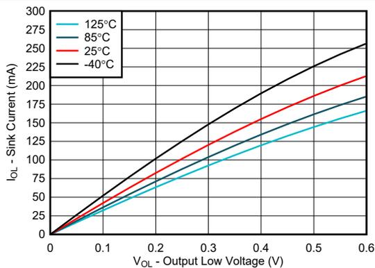
Figure 5-9. I/O Sink Current vs Output Low Voltage, V<sub>CCP</sub> = 2.5 V
