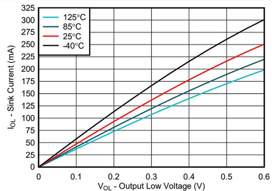
Figure 5-10. I/O Sink Current vs Output Low Voltage, V<sub>CCP</sub> = 3.3 V
