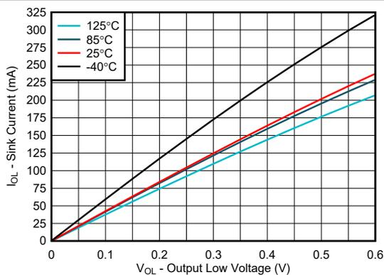
Figure 5-11. I/O Sink Current vs Output Low Voltage, V<sub>CCP</sub> = 3.6 V
