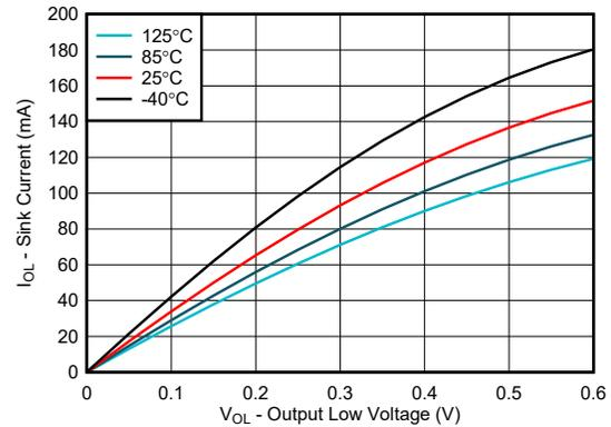
Figure 5-8. I/O Sink Current vs Output Low Voltage, V<sub>CCP</sub> = 1.8 V
