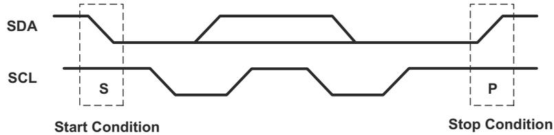
**Figure 7-4. Definition of Start and Stop Conditions**
