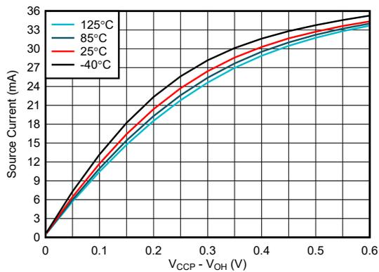
Figure 5-13. I/O Source Current vs Output High Voltage, V<sub>CCP</sub> = 1.08 V
