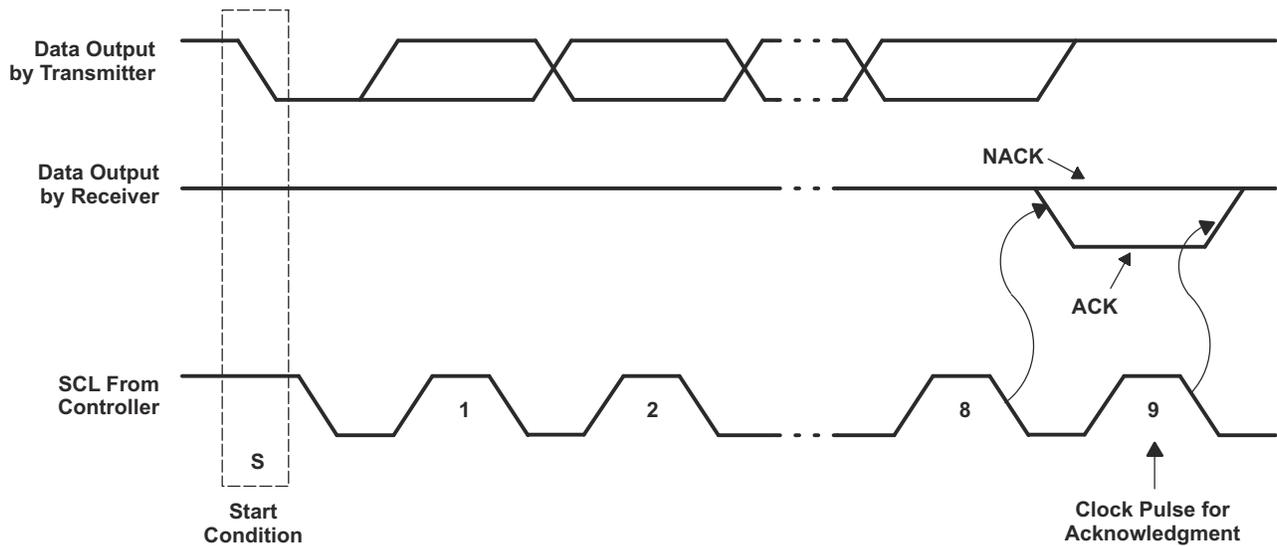
**Figure 7-6. Acknowledgment on the I<sup>2</sup>C Bus**
