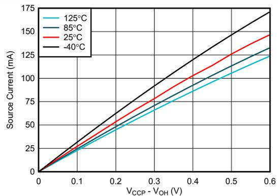
Figure 5-16. I/O Source Current vs Output High Voltage, V<sub>CCP</sub> = 2.5 V
