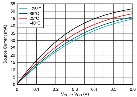
Figure 5-14. I/O Source Current vs Output High Voltage, V<sub>CCP</sub> = 1.2 V
