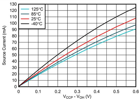
Figure 5-15. I/O Source Current vs Output High Voltage, V<sub>CCP</sub> = 1.8 V
