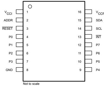
**Figure 4-1. PW (TSSOP) Package, 16-Pin (Top View)**
