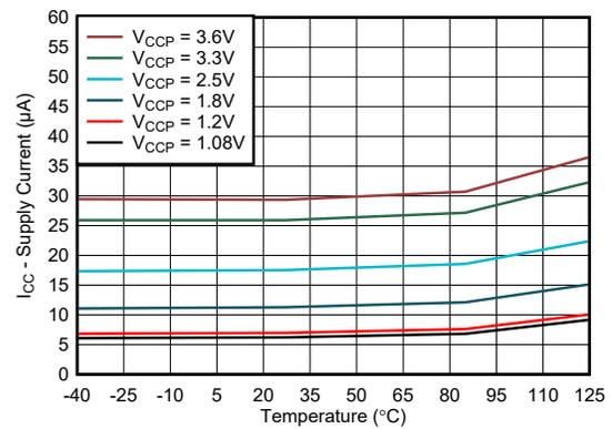
Figure 5-2. Supply Current vs Temperature - FM+ mode
