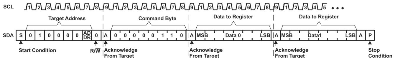
**Figure 7-10. Write to Configuration or Polarity Inversion Registers**
