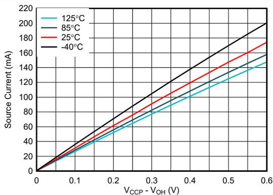
Figure 5-17. I/O Source Current vs Output High Voltage, V<sub>CCP</sub> = 3.3 V
