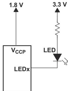
**Figure 8-3. Device Supplied by a Lower Voltage**
