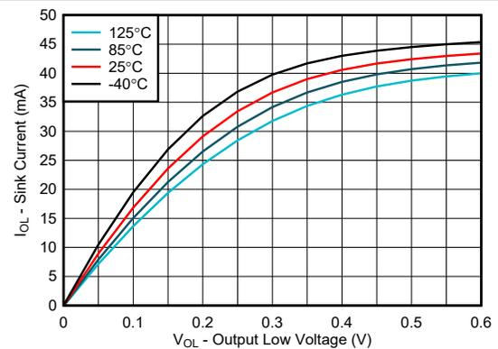
Figure 5-6. I/O Sink Current vs Output Low Voltage, V<sub>CCP</sub> = 1.08 V
