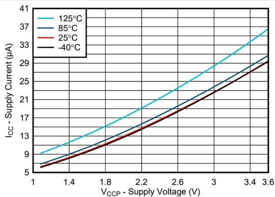
Figure 5-5. Supply Current vs Supply Voltage - FM+ mode
