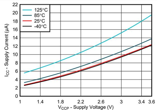
Figure 5-4. Supply Current vs Supply Voltage - FM mode
