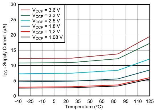
Figure 5-1. Supply Current vs Temperature - FM mode
