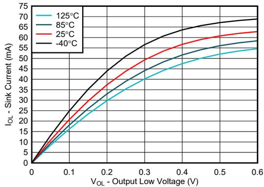
Figure 5-7. I/O Sink Current vs Output Low Voltage, V<sub>CCP</sub> = 1.2 V
