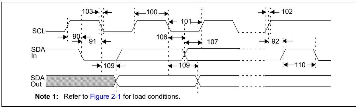
**FIGURE 2-6:** I<sup>2</sup>C™ Bus Data Timing.
