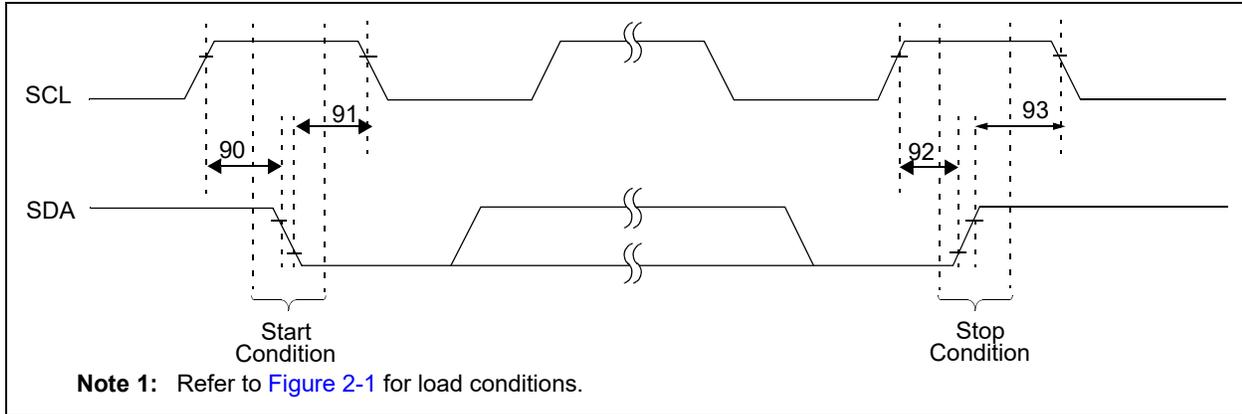
**FIGURE 2-5:** I<sup>2</sup>C™ Bus Start/Stop Bits Timing.
