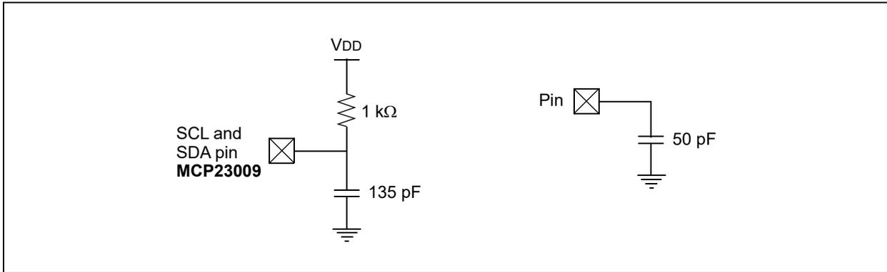
**FIGURE 2-1:** Load Conditions for Device Timing Specifications.
