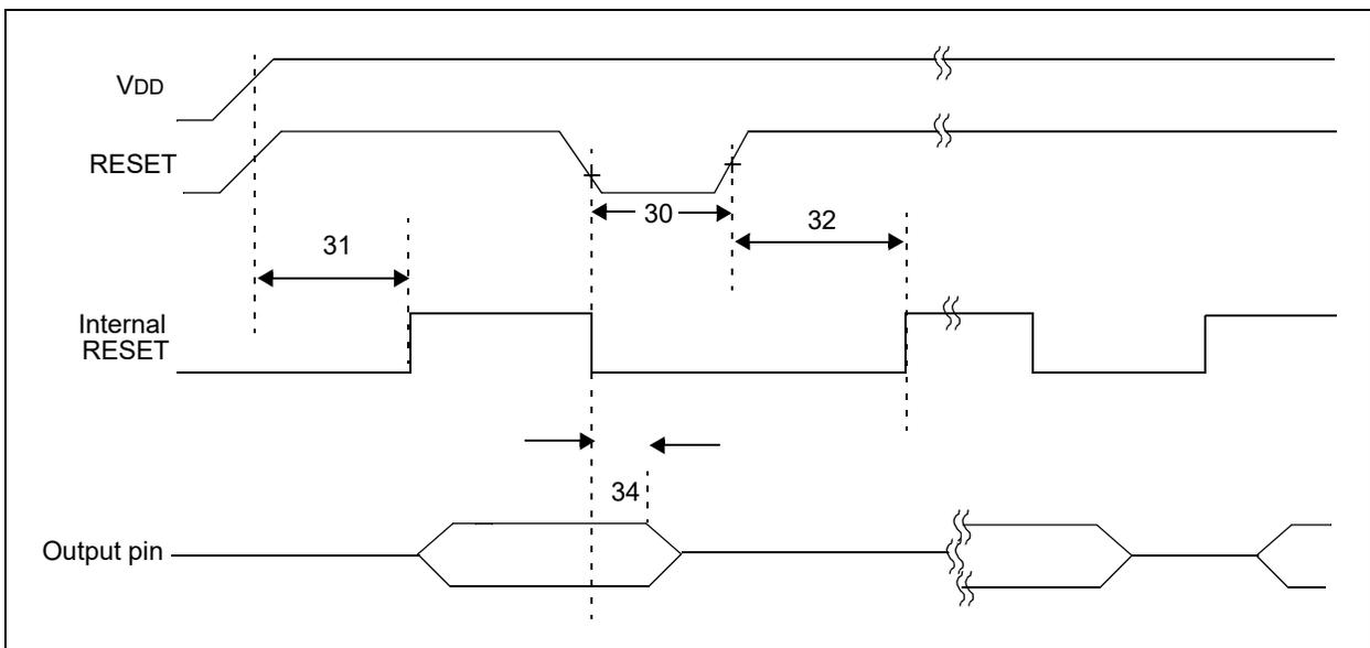
**FIGURE 2-2:** RESET and Device Reset Timer Timing.
