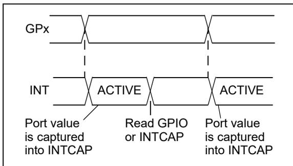
**FIGURE 1-11:** *Interrupt-on-Pin-Change.*
