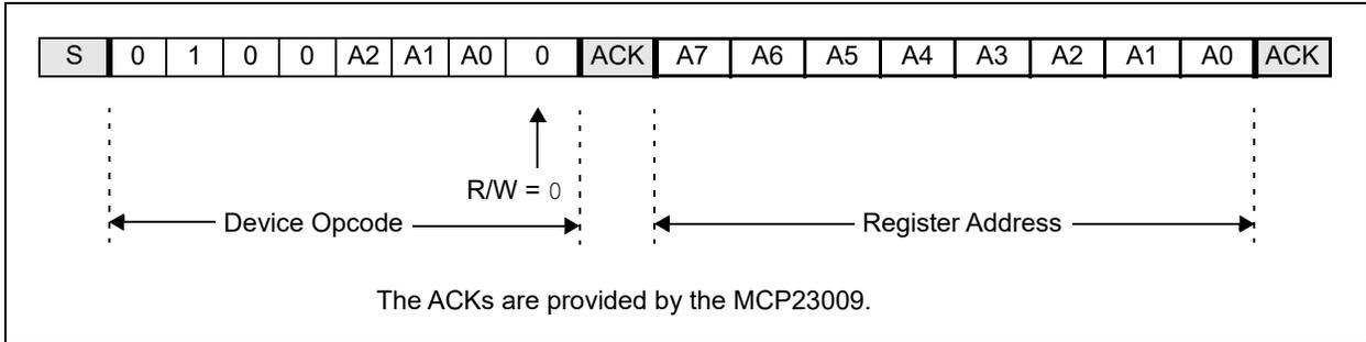
**FIGURE 1-8:** I<sup>2</sup>C™ Addressing Registers.
