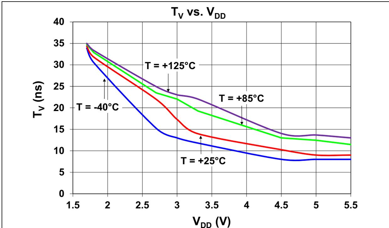
**FIGURE 2-9:** Typical Performance Curve for SPI T<sub>V</sub> Specification (Param #12).
