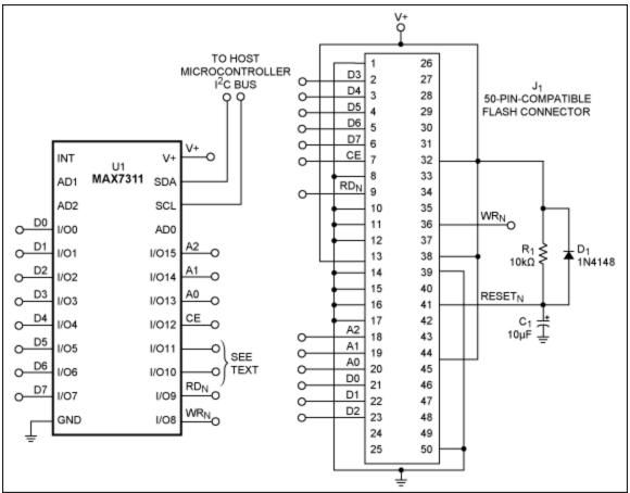
Figure 1. This circuit employs a 16-bit I/O extender (the MAX7311) to connect a compact flash connector to the I<sup>2</sup>C bus of a microcontroller.
