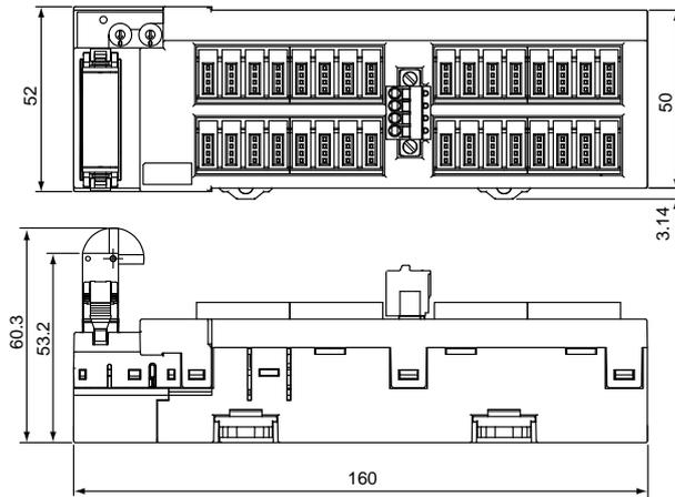
Digital I/O Slave Units with e-CON Connector (Vertical type)
