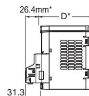
Note. After the CompoNet Communication Unit is installed, dimension D of the inverter increases by 26.4 mm. (Dimension D of the inverter varies depending on the capacity. Refer to the MX2-series USER'S MANUAL(Cat.No.I570))
