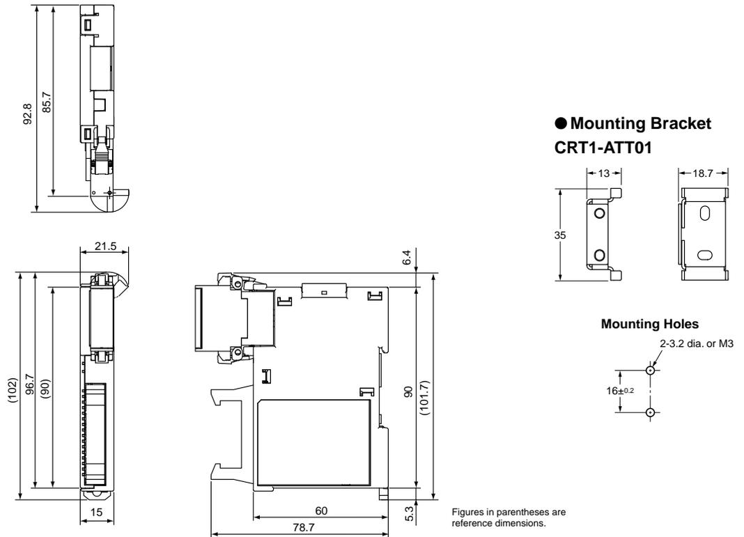
Digital I/O Slave Units with MIL Connector (Vertical type)
