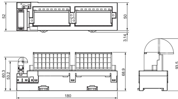
Digital I/O Slave Units with e-CON Connectors
