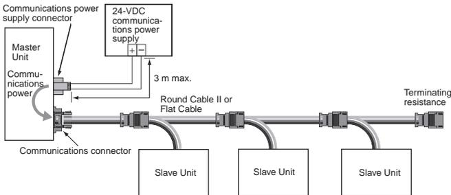
When Repeater Units are used, communications power to sub-trunk lines is supplied by the downstream port communications power supply connectors (BS+ and BS-) of the Repeater Units. The cable between the communications power supply and the communications power supply connector must be no longer than 3 m.
