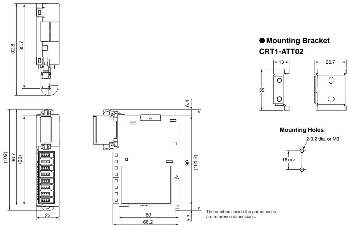
Digital I/O Slave Units with MIL Connector (Vertical type)
