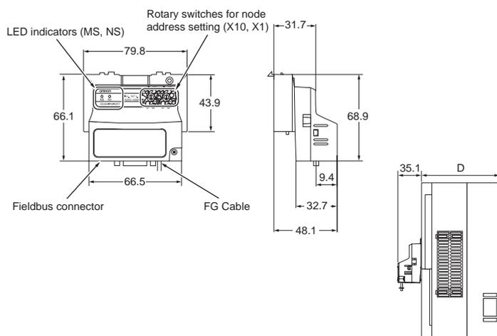
**Note.** After the CompoNet Communication Unit is installed, dimension D of the inverter increases by 35.1 mm. (Dimension D of the inverter varies depending on the capacity. Refer to the RX-Series V1 type USER'S MANUAL(Cat.No.I578))
