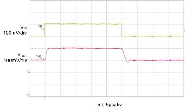
**Figure 5. Test Result with R<sub>NULL</sub> 330Ω**
