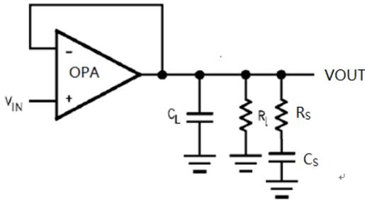
**Figure 6. The RC Snubber Circuit**
