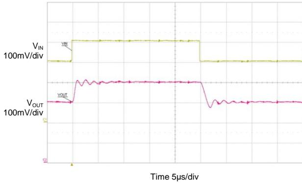
**Figure 4. Test Result Without R<sub>NULL</sub>**
