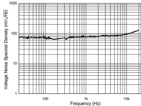
Figure 2. Input Voltage Noise in Zero-Drift Amplifier
