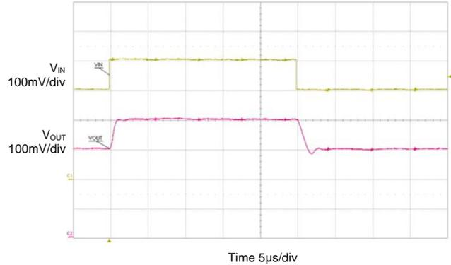
**Figure 5. Test Result with R<sub>NULL</sub> 330Ω**
