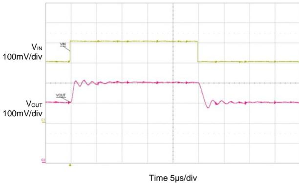
**Figure 4. Test Result Without R<sub>NULL</sub>**
