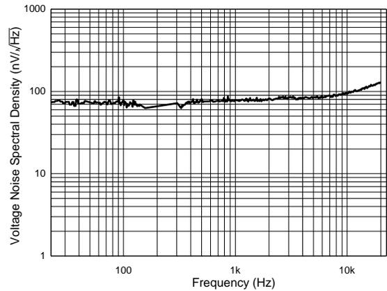
Figure 2. Input Voltage Noise in Zero-Drift Amplifier (AS2333)
