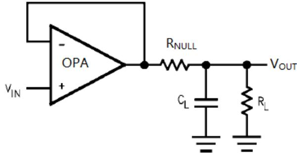
**Figure 3. Capacitive Load with R<sub>NULL</sub>**
