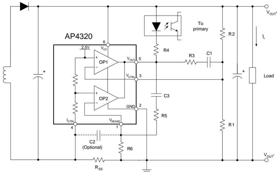
$$V_{OUT} = V_{REF} \times \frac{R1 + R2}{R1}$$
