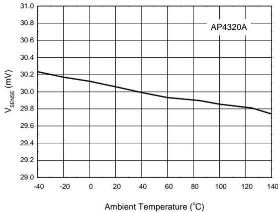
**V<sub>SENSE</sub> vs. Ambient Temperature**
