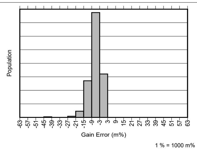
Figure 7-12. All Gains INA241B Gain Error Production Distribution
