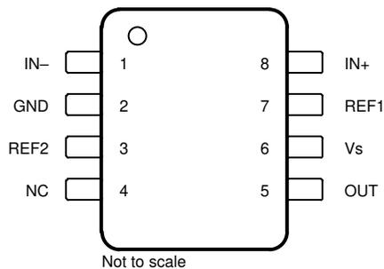
**Figure 6-1. INA241x: DDF Package 8-Pin SOT-23 Top View**
