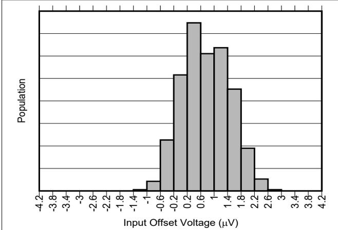
**Figure 7-3. INA241A3 and INA241A4 Input Offset Production Distribution**
