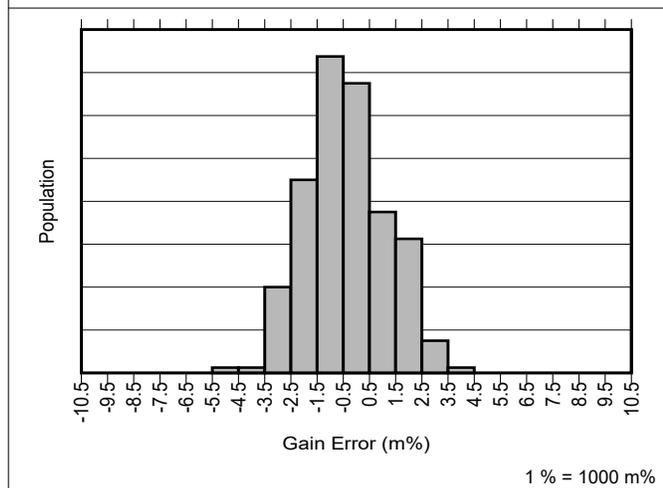
Figure 7-11. INA241A4 and INA241A5 Gain Error Production Distribution
