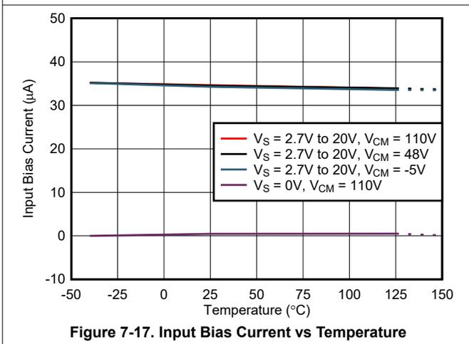
Figure 7-17. Input Bias Current vs Temperature
