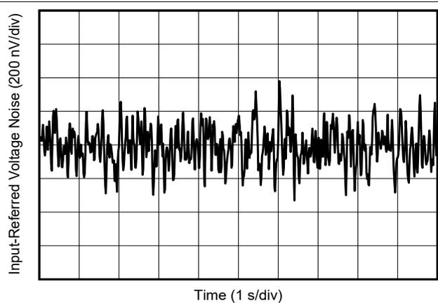
Figure 7-28. 0.1 Hz to 10 Hz Voltage Noise
