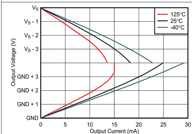
Figure 7-23. Output Voltage vs Output Current
