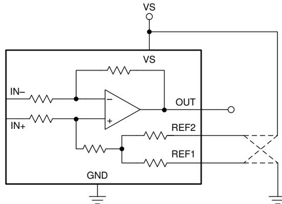
**Figure 8-2. Test Circuit For Reference Divider Accuracy**
