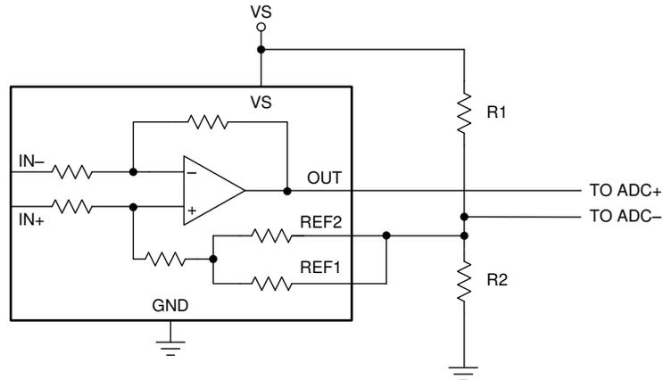
**Figure 8-8. Setting the Reference Using a Resistor Divider**
