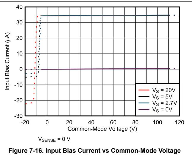
Figure 7-16. Input Bias Current vs Common-Mode Voltage
