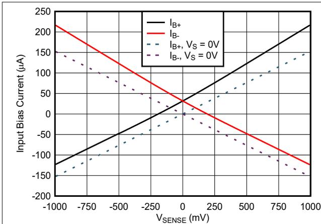
Figure 7-19. INA241x2 Input Bias Current vs  $V_{\text{SENSE}}$
