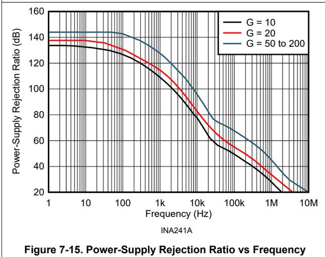
Figure 7-15. Power-Supply Rejection Ratio vs Frequency
