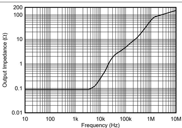
Figure 7-24. Output Impedance vs Frequency
