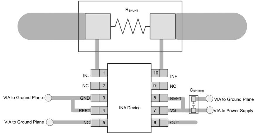
**Figure 9-4. INA241x 10-Pin VSSOP (DGS) Package Recommended Layout**
