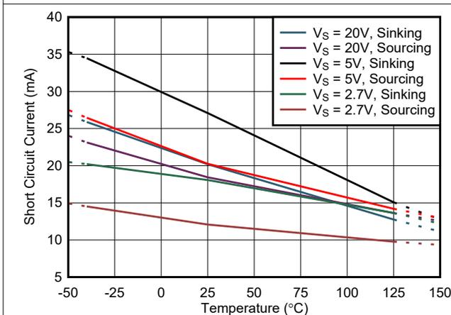
Figure 7-29. Short-Circuit Current vs Temperature
