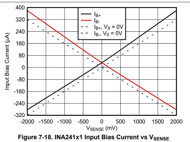
Figure 7-18. INA241x1 Input Bias Current vs  $V_{\text{SENSE}}$
