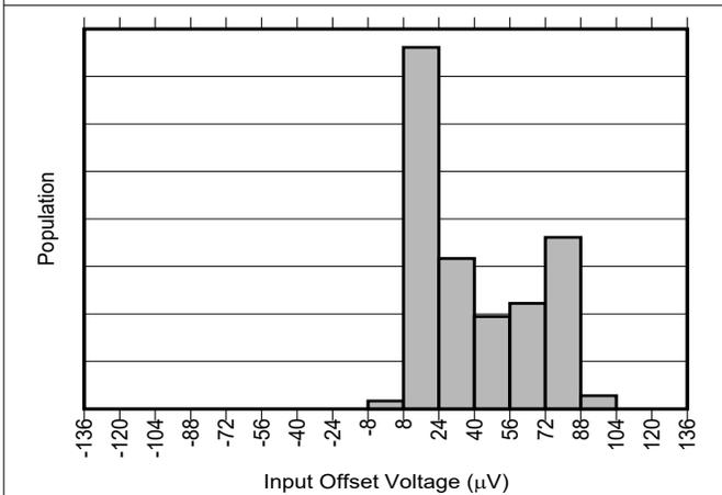
**Figure 7-5. All Gains INA241B Input Offset Production Distribution**
