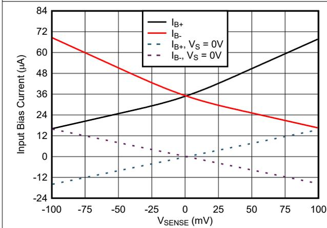
Figure 7-21. INA241x5 Input Bias Current vs  $V_{\text{SENSE}}$
