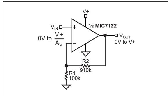
**FIGURE 3-3:** Non-Inverting Amplifier.
