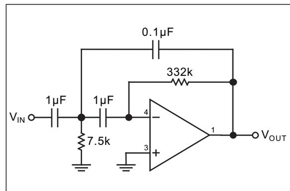
FIGURE 4-4: High-Pass Filter.
