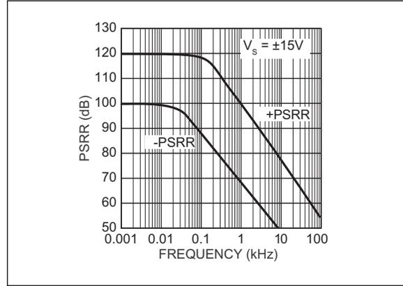
**FIGURE 2-9:** Power Supply Rejection Ratio vs. Frequency.
