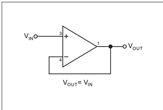
FIGURE 4-1: Voltage Buffer.
