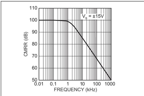
**FIGURE 2-8:** Common Mode Rejection Ratio vs. Frequency.
