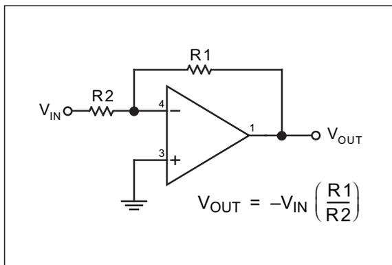
FIGURE 4-2: Inverting Amplifier.
