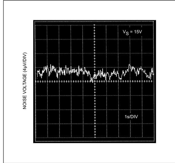
**FIGURE 2-13:** 0.1 Hz to 10 Hz Noise.
