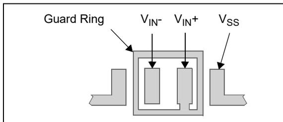
**FIGURE 4-6:** Example Guard Ring Layout for Inverting Gain.
