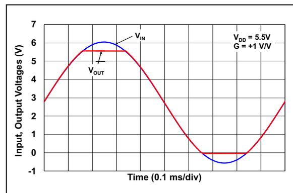
**FIGURE 2-37:** The MCP6476/6R/6U/7/9 Device Shows No Phase Reversal.
