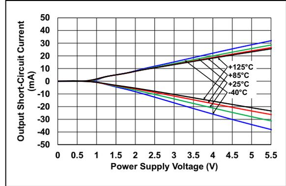
**FIGURE 2-15:** Output Short-Circuit Current vs. Power Supply Voltage.
