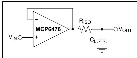
FIGURE 4-5: Output Resistor,  $R_{ISO}$ , Stabilizes Large Capacitive Loads.
