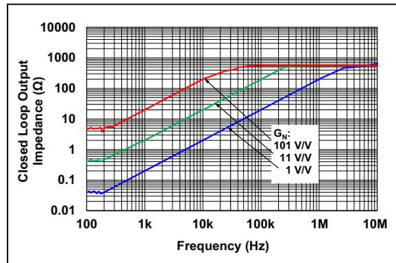
**FIGURE 2-22:** Closed Loop Output Impedance vs. Frequency.
