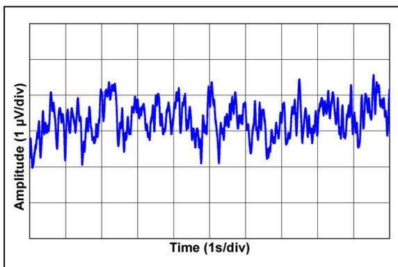
**FIGURE 2-29:** 0.1 Hz to 10 Hz Voltage Noise.
