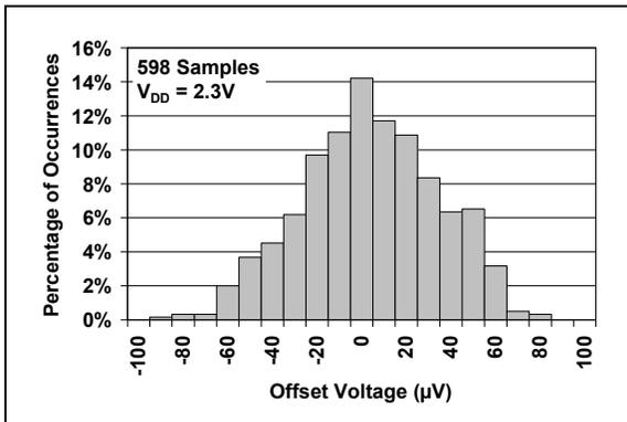
**FIGURE 2-2:** Input Offset Voltage at  $V_{DD} = 2.3V$ .
