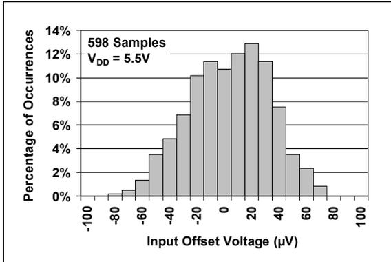
**FIGURE 2-1:** Input Offset Voltage at  $V_{DD} = 5.5V$ .
