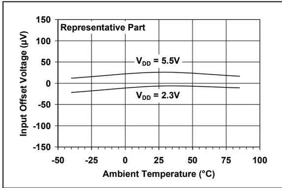
**FIGURE 2-7:** Input Offset Voltage vs. Ambient Temperature.
