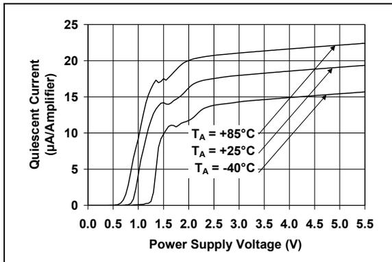
**FIGURE 2-19:** Quiescent Current vs. Power Supply Voltage.
