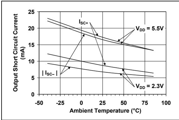
**FIGURE 2-13:** Output Short Circuit Current vs. Ambient Temperature.
