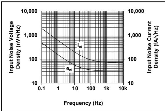
**FIGURE 2-26:** Input Noise Voltage, Current Densities vs. Frequency.
