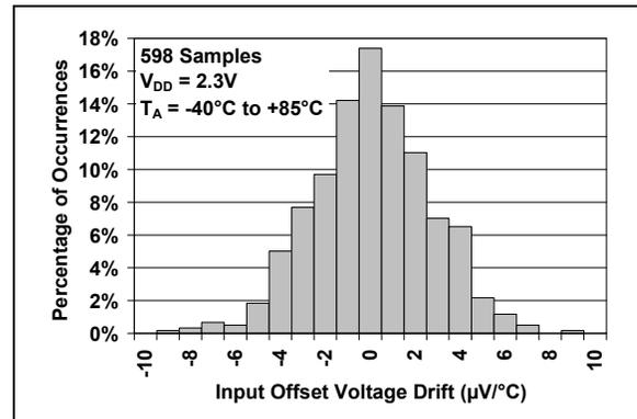
**FIGURE 2-5:** Input Offset Voltage Drift at  $V_{DD} = 2.3V$ .
