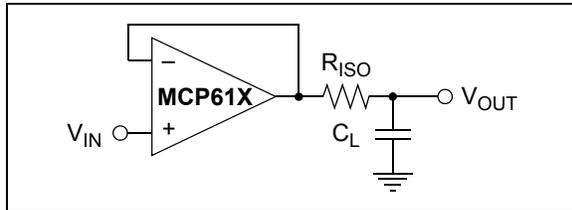
**FIGURE 4-5:** Output Resistor,  $R_{ISO}$  stabilizes large capacitive loads.
