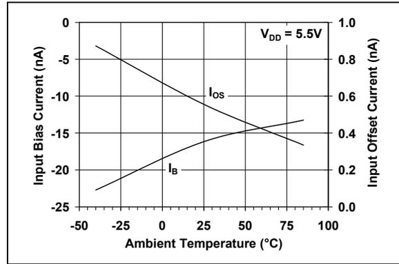
**FIGURE 2-10:** Input Bias, Offset Currents vs. Ambient Temperature.
