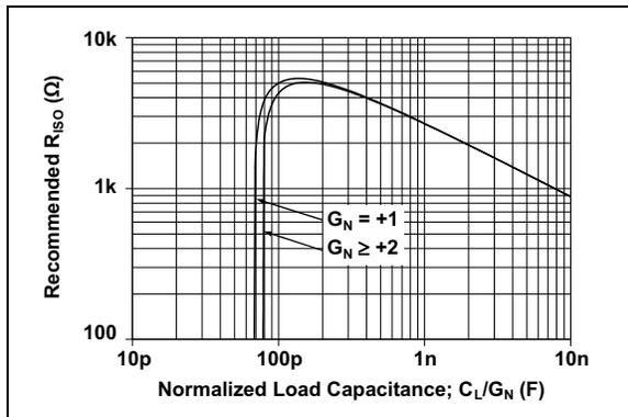
**FIGURE 4-6:** Recommended  $R_{ISO}$  Values for Capacitive Loads.
