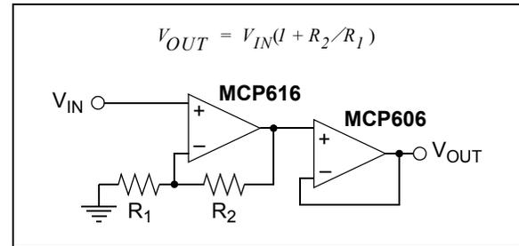
**FIGURE 4-12:** Precision Gain with Good Load Isolation.
