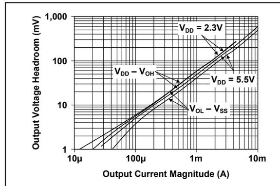
**FIGURE 2-22:** Output Voltage Headroom vs. Output Current Magnitude.
