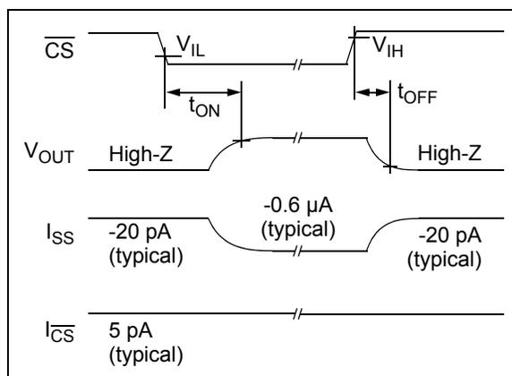
**FIGURE 1-1:** Chip Select ( $\overline{\text{CS}}$ ) Timing Diagram (MCP6043 only).
