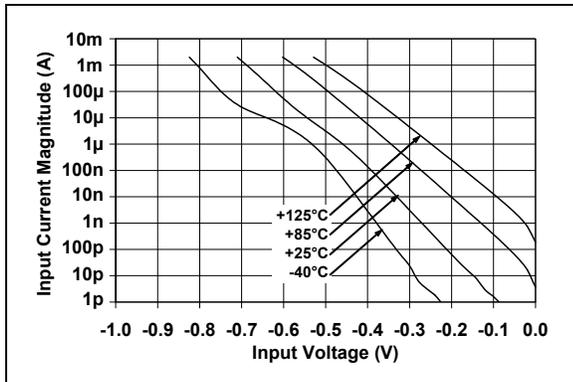
**FIGURE 2-33:** Input Current vs. Input Voltage (below  $V_{SS}$ ).
