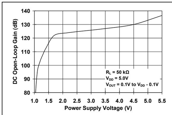
**FIGURE 2-15:** DC Open-Loop Gain vs. Power Supply Voltage.
