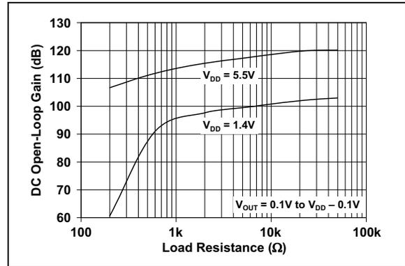
**FIGURE 2-17:** DC Open-Loop Gain vs. Load Resistance.
