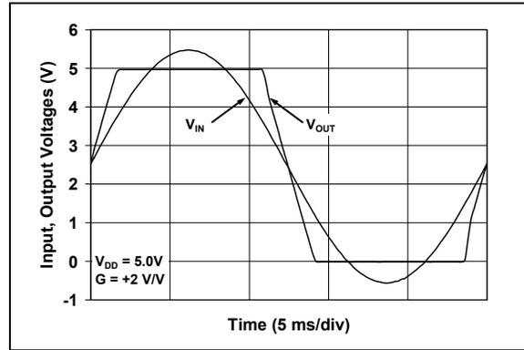
**FIGURE 2-10:** The MCP6041/2/3/4 family shows no phase reversal.
