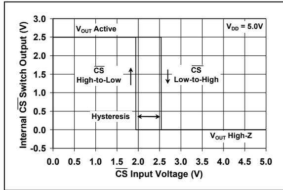
**FIGURE 2-35:** Chip Select ( $\overline{\text{CS}}$ ) Hysteresis (MCP6043 only).
