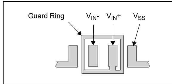
FIGURE 4-6: Example Guard Ring Layout for Inverting Gain.
