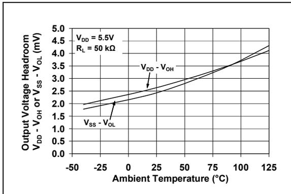
**FIGURE 2-26:** Output Voltage Headroom vs. Ambient Temperature.
