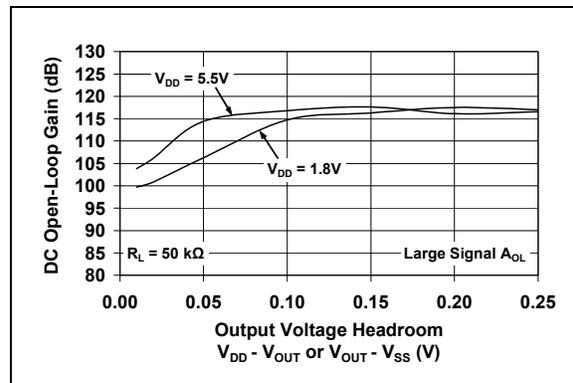
**FIGURE 2-18:** DC Open-Loop Gain vs. Output Voltage Headroom.
