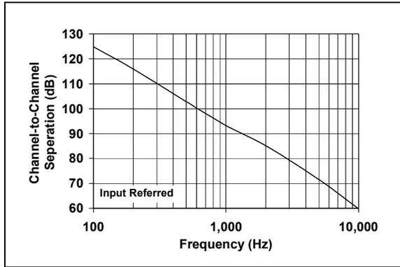
**FIGURE 2-19:** Channel-to-Channel Separation vs. Frequency (MCP6032/4 only).
