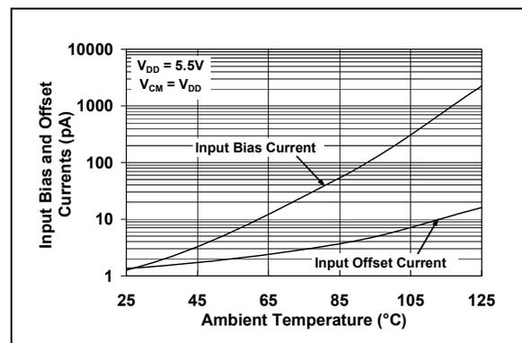
**FIGURE 2-11:** Input Bias, Offset Currents vs. Ambient Temperature.
