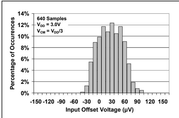
**FIGURE 2-1:** Input Offset Voltage with  $V_{DD} = 3.0\text{V}$ .
