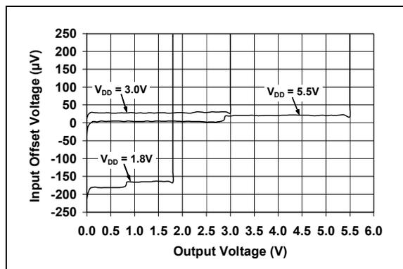
**FIGURE 2-6:** Input Offset Voltage vs. Output Voltage.
