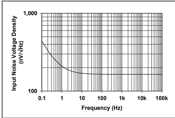
**FIGURE 2-7:** Input Noise Voltage Density vs. Frequency.
