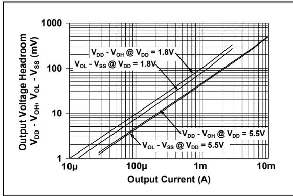
**FIGURE 2-25:** Output Voltage Headroom vs. Output Current.
