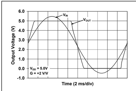
**FIGURE 2-32:** The MCP6031/2/3/4 Family Shows No Phase Reversal.
