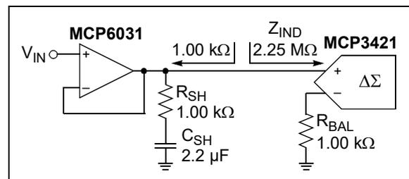
**FIGURE 4-9:** Driving the MCP3421 Using an R-C Snubber.
