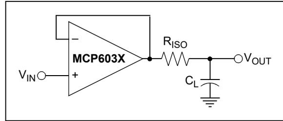
**FIGURE 4-3:** Output Resistor,  $R_{ISO}$ , Stabilizes Large Capacitive Loads.
