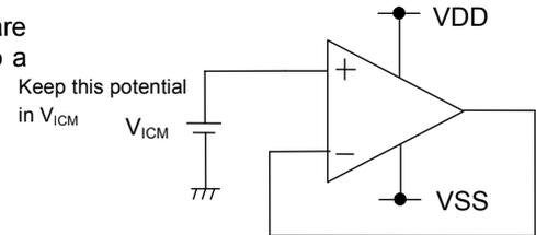
Figure 56. Example of Application Circuit for Unused Op-amp
