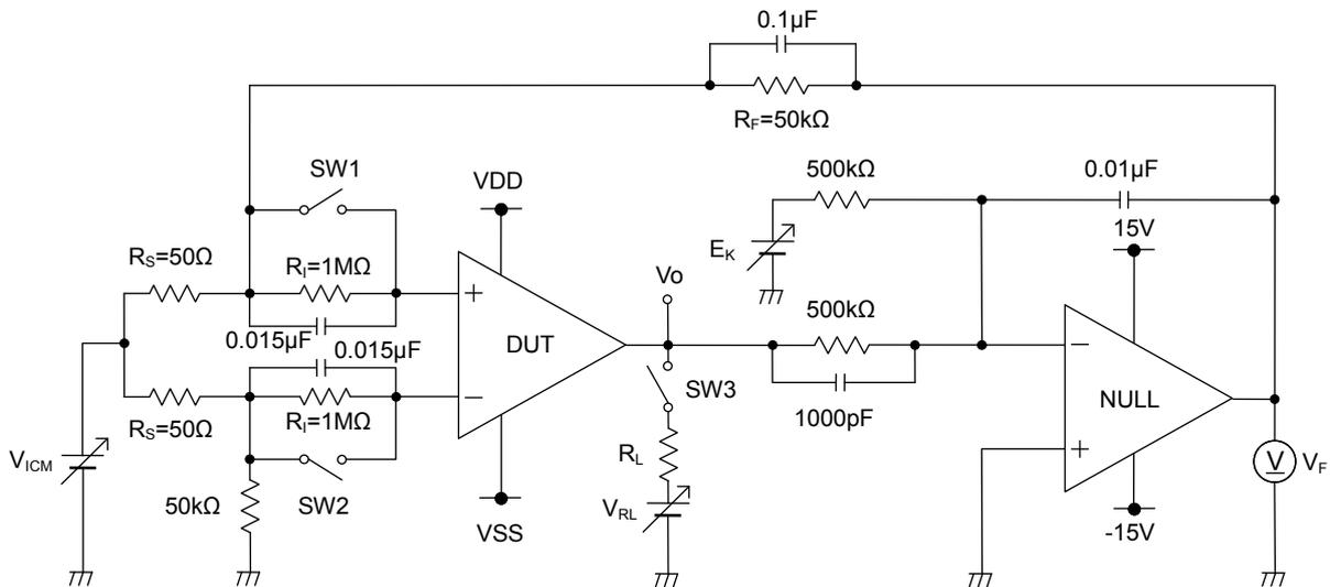
Figure 48. Test Circuit 1 (one channel only)
