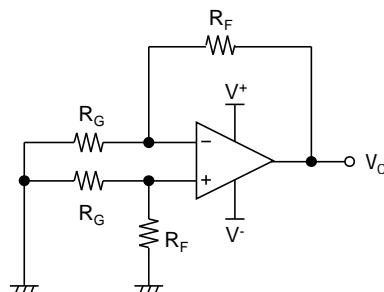
$$V_{IO} = \frac{R_G}{(R_G + R_F)} \times V_0$$
