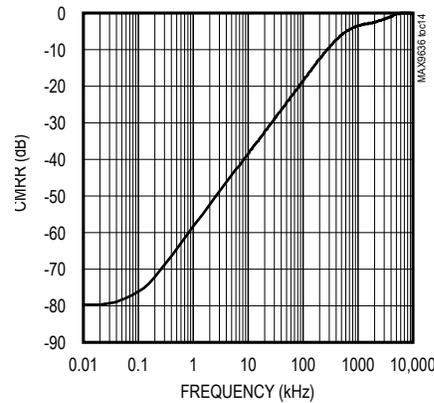
DC COMMON-MODE REJECTION RATIO
