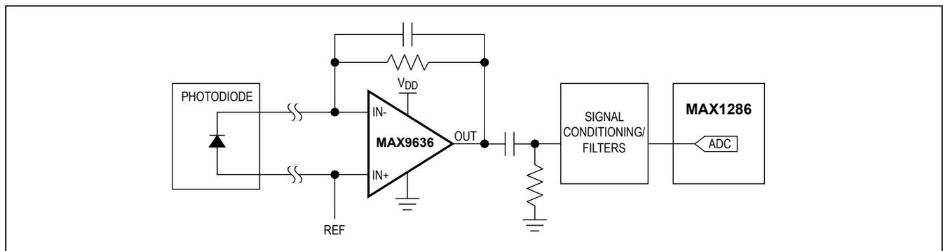
Figure 3. The MAX9636 in a Sensor Preamp Configuration
