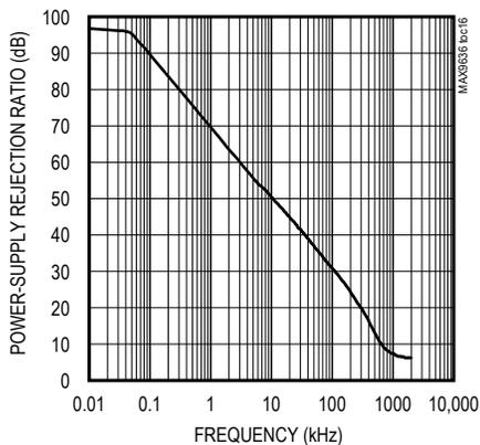
DC POWER-SUPPLY REJECTION RATIO
