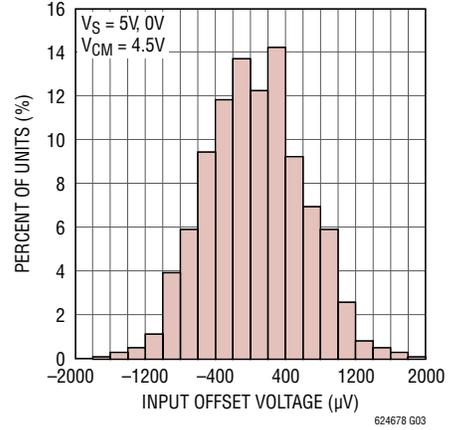
**$V_{OS}$  Distribution,  $V_{CM} = V^+ - 0.5\text{V}$
