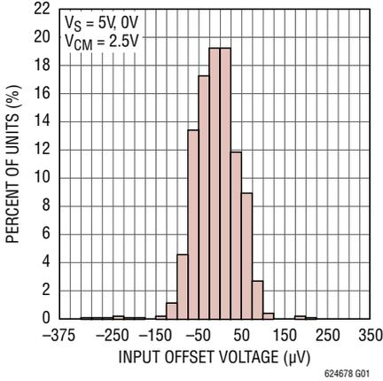
**$V_{OS}$  Distribution,  $V_{CM} = V_S/2$
