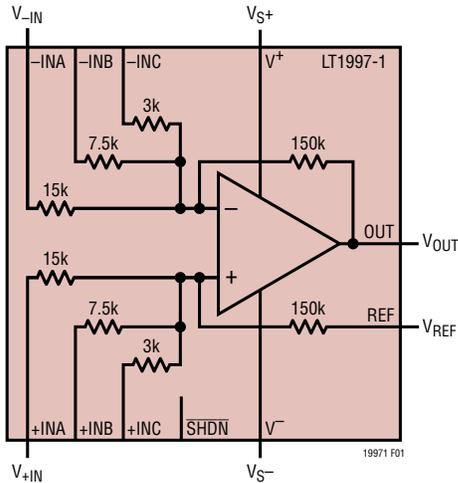
**Figure 1. Difference Amplifier with Dual-Supply Operation (Gain = 10)**
