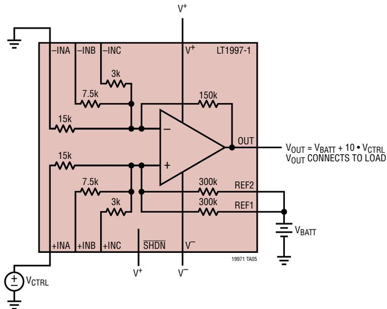
THIS CIRCUIT USES A GROUND-REFERENCED CONTROL SIGNAL TO CREATE A SUPPLY ON TOP OF AN EXISTING SUPPLY ( $V_{BATT}$ )
