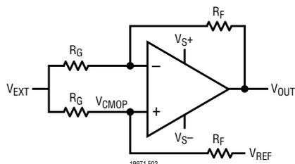
**Figure 2. Calculating the Common Mode Input Voltage Range**
