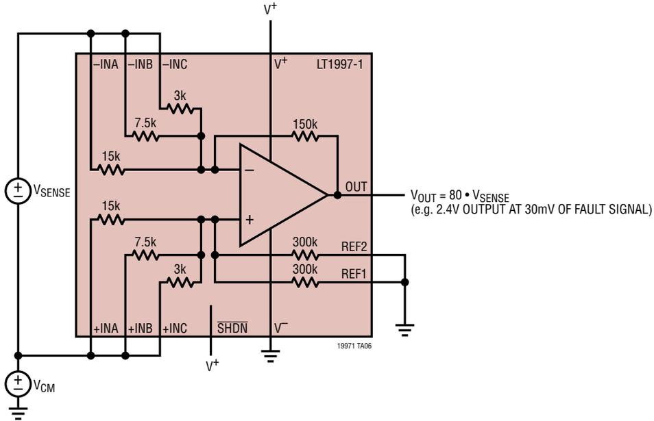
FAULT DETECTION AT HIGH COMMON MODE VOLTAGE: LOOK FOR AN INCREASING VOLTAGE THAT MIGHT INDICATE BREAKAGE.
