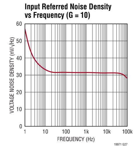
**TYPICAL PERFORMANCE CHARACTERISTICS**  $T_A = 25^\circ\text{C}$ ,  $V_S = \pm 15\text{V}$ , Difference Amplifier configuration, unless otherwise noted.
