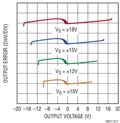
**Typical Gain Error for  $R_L = 2\text{k}\Omega$  (G = 10) (Curves Offset for Clarity)**
