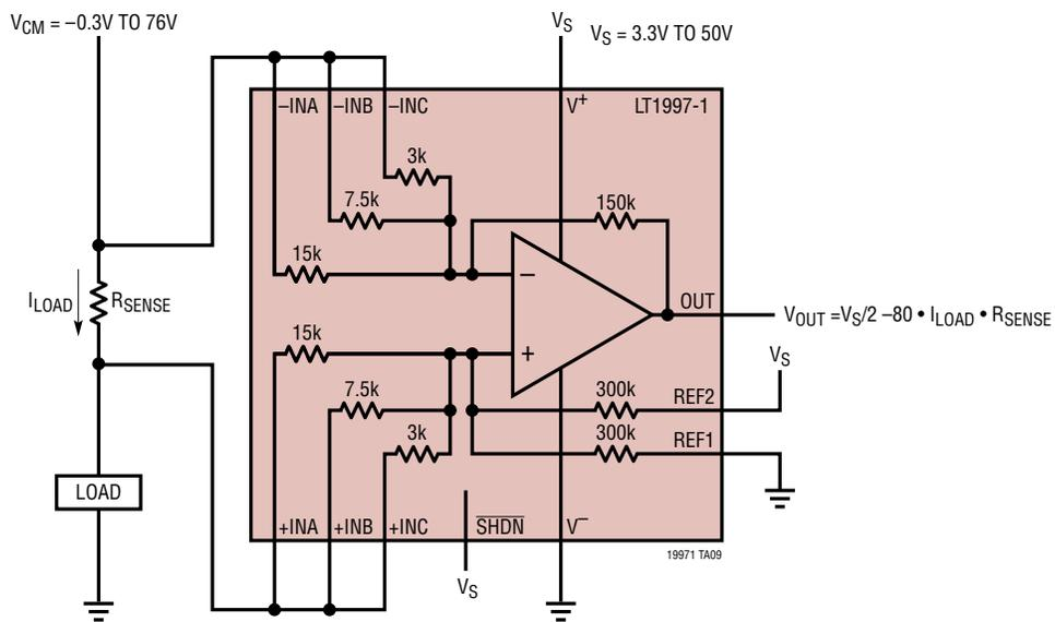
OUTPUT OFFSET INCREASES WHEN  $V_{CM} > V_S$
