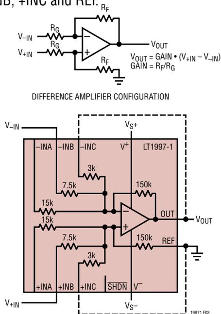
DIFFERENCE AMPLIFIER CONFIGURATION IMPLEMENTED WITH THE LT1997-1,  $R_{\text{F}} = 150\text{k}$ ,  $R_{\text{G}} = 7.5\text{k}$ , GAIN = 20
