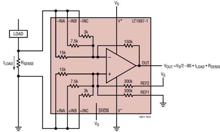
THIS CIRCUIT PROVIDES BIDIRECTIONAL LOW SIDE CURRENT SENSE BECAUSE IT CAN WORK AT SLIGHTLY NEGATIVE VOLTAGES ON THE -INA/-INB/-INC INPUT PINS, AS DRAWN
