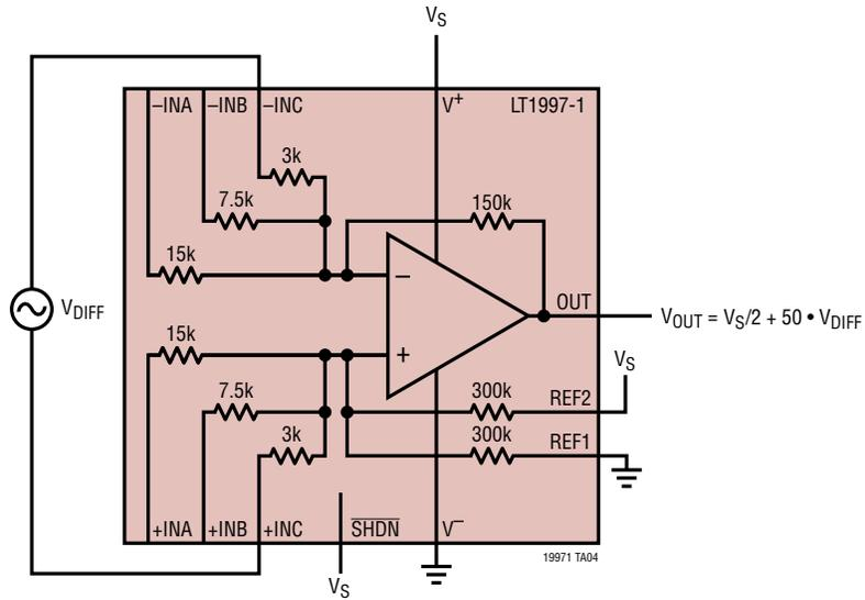
THE INPUT SIGNAL FLOATS. THE VOLTAGE AT THE REF INPUTS AND THE OUTPUT VOLTAGE DETERMINE THE COMMON MODE VOLTAGE AT THE INPUT
