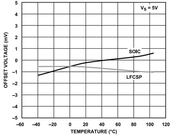
Figure 41. Offset Voltage vs. Temperature ( $V_S = 5V$ )
