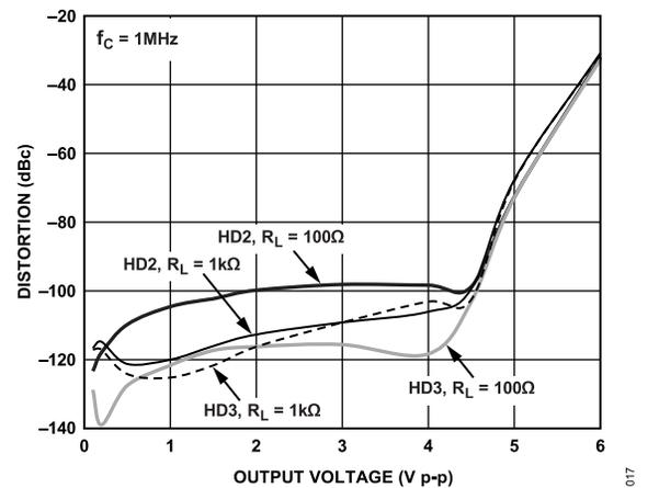
Figure 19. Distortion vs. Output Voltage for Various Loads
