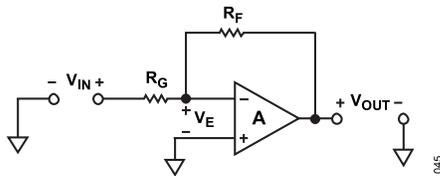
Figure 53. Inverting Configuration
