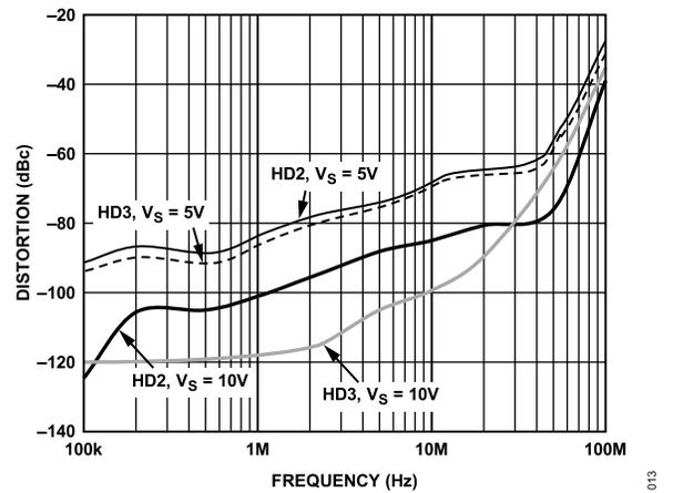
Figure 18. Distortion vs. Frequency for Various Supplies, V<sub>OUT</sub> = 2 V p-p
