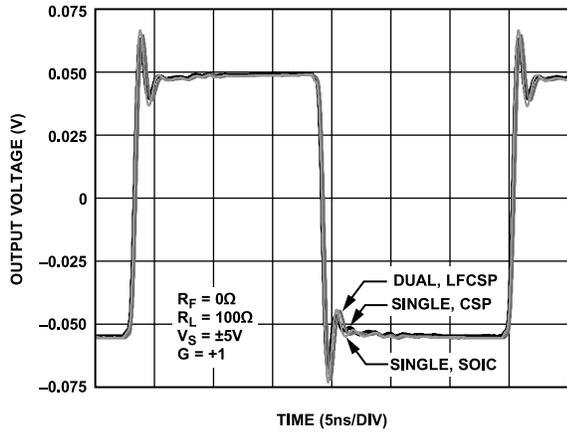
Figure 20. Small Signal Transient Response vs. Package
