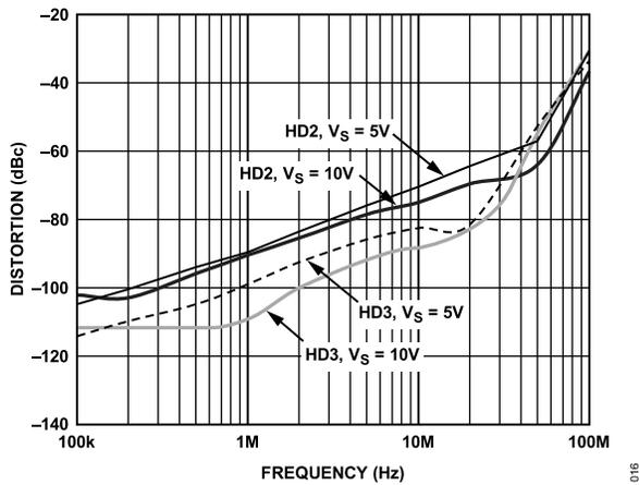
Figure 16. Distortion vs. Frequency for Various Supplies, G = 2, V<sub>OUT</sub> = 2 V p-p
