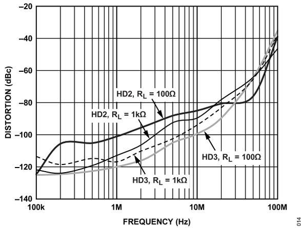
Figure 15. Distortion vs. Frequency for Various Loads, V<sub>OUT</sub> = 2 V p-p
