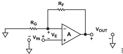
Figure 52. Noninverting Configuration
