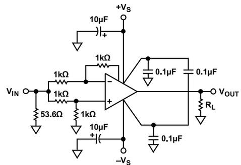
Figure 51. Common-Mode Rejection
