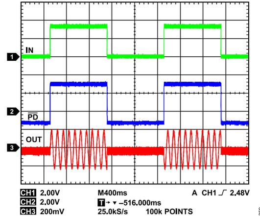
**Figure 58. Power-Down Operation**
