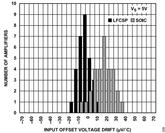
Figure 42. Input Offset Voltage Drift Histogram ( $V_S = 5V$ )
