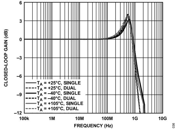
Figure 17. Small Signal Frequency Response vs. Temperature
