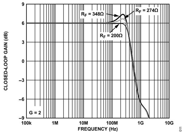
Figure 13. Small Signal Frequency Response for Various  $R_F$
