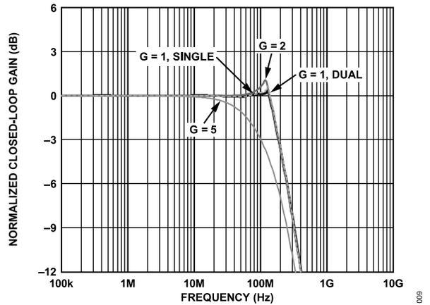
Figure 11. Large Signal Frequency Response for Various Gains
