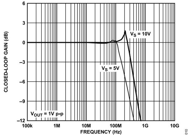
Figure 12. Large Signal Frequency Response for Various Supplies
