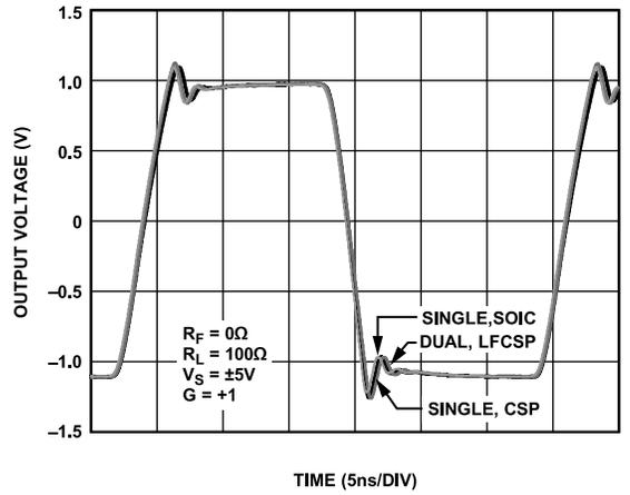
Figure 23. Large Signal Transient Response vs. Package
