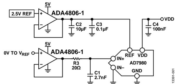
Figure 1. Driving the AD7980 with the ADA4806-1
