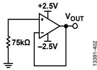
Figure 48. Current Noise Test Circuit (See Figure 20)
