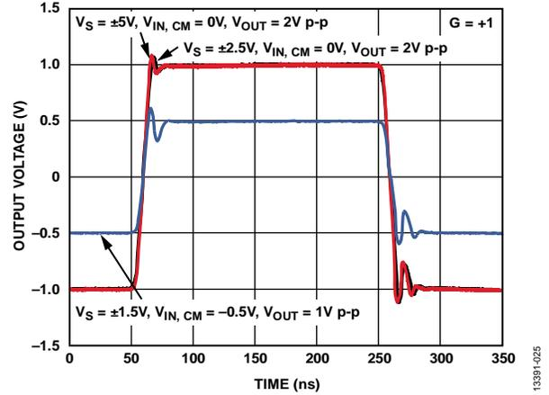
Figure 32. Large Signal Transient Response for Various Supplies
