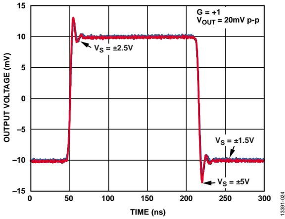
Figure 29. Small Signal Transient Response for Various Supplies
