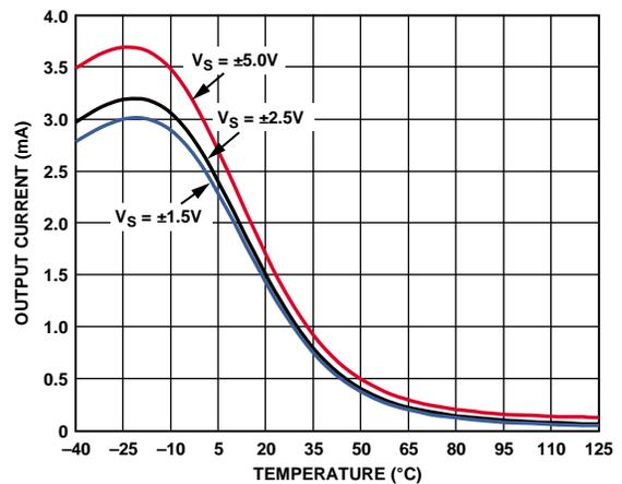
Figure 45. Sleep Mode Output Current vs. Temperature
