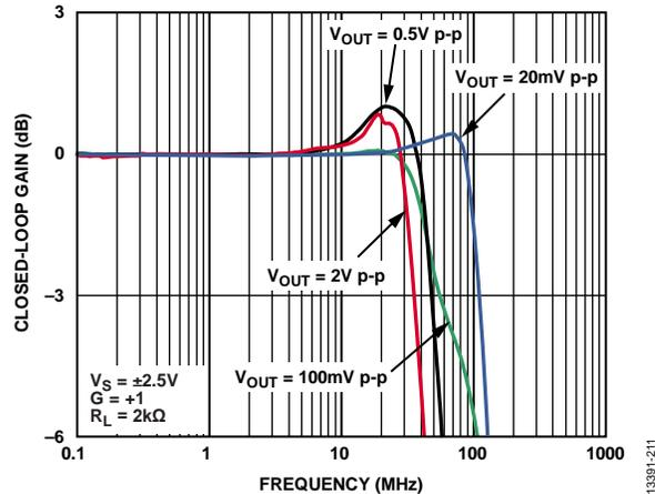
Figure 10. Frequency Response for Various Output Voltages
