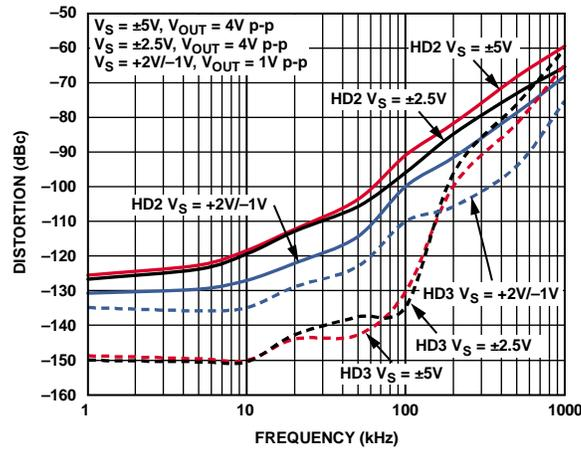
Figure 16. Distortion vs. Frequency, G = +2
