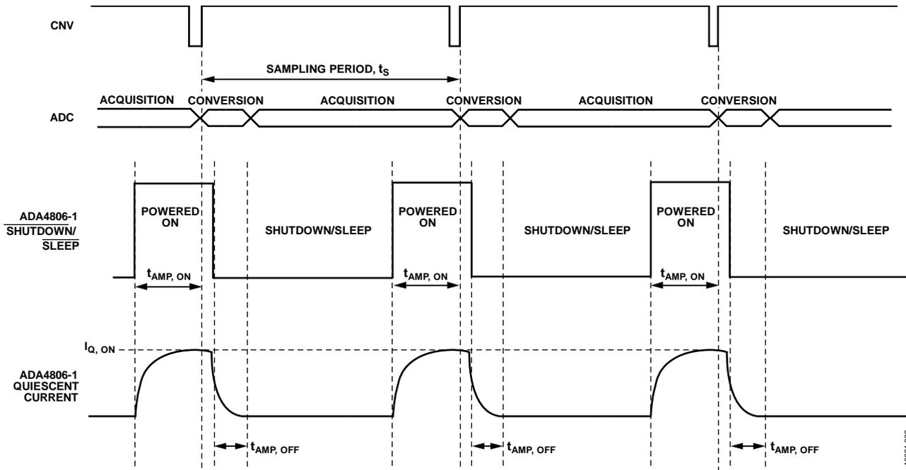
Figure 63. Timing Waveforms
