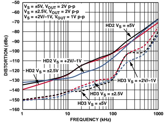
Figure 15. Distortion vs. Frequency for Various Supplies, G = +1
