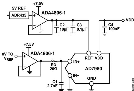
Figure 61. Driving the AD7980 with the ADA4806-1
