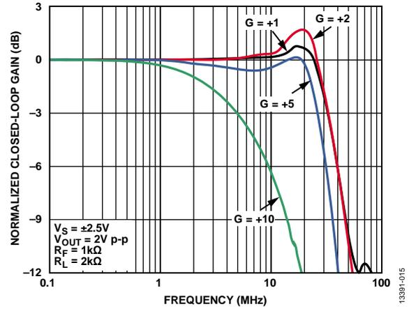
Figure 8. Large Signal Frequency Response for Various Gains
