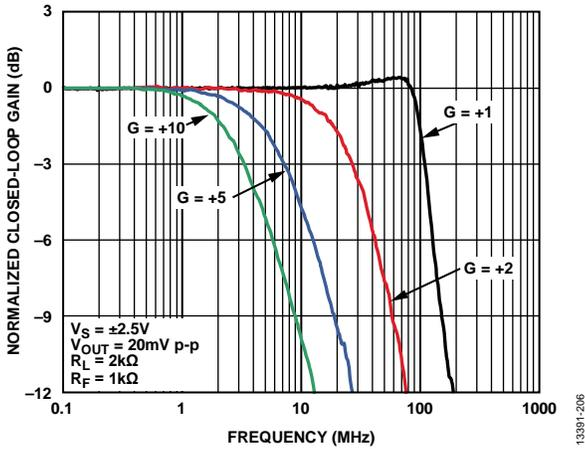
Figure 5. Small Signal Frequency Response for Various Gains
