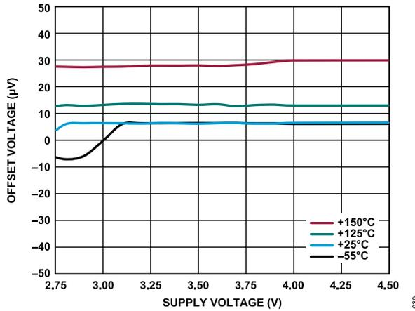
Figure 32. Offset Voltage vs. Minimum Supply Voltage
