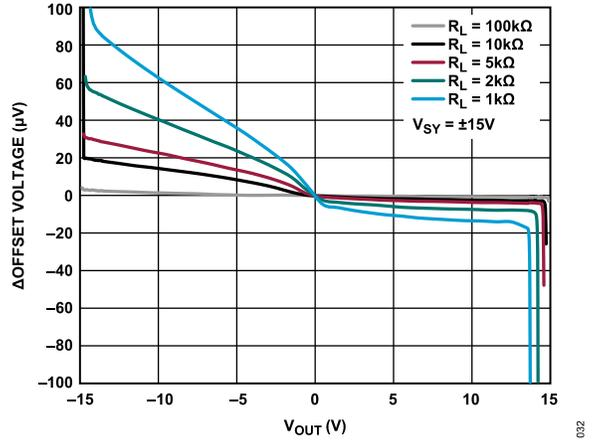
Figure 34. ΔOffset Voltage vs.  $V_{OUT}$
