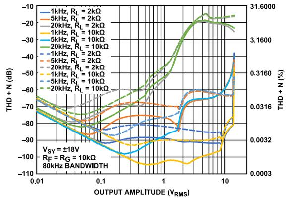
Figure 47. THD + N vs. Output Amplitude
