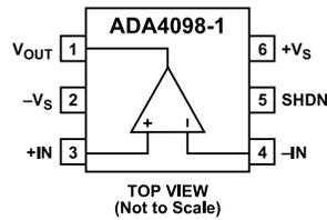
Figure 4. Pin Configuration for ADA4098-1 6-Lead TSOT
