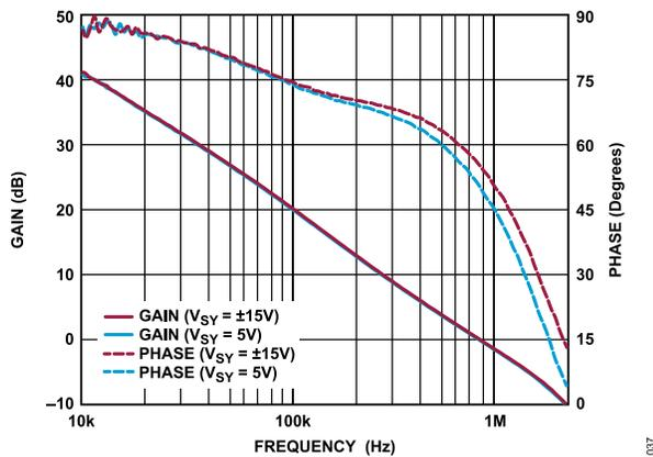
Figure 39. Loop Gain and Phase vs. Frequency
