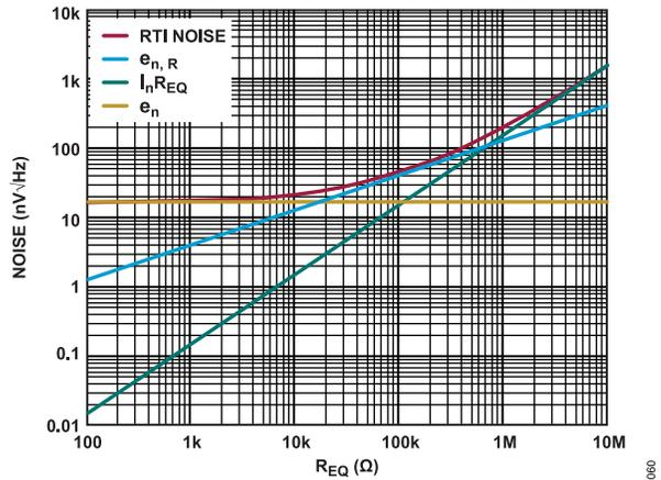
Figure 61. Noise Contributions vs. Equivalent Input Resistance
