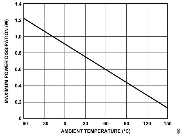
Figure 3. Maximum Power Dissipation vs. Ambient Temperature
