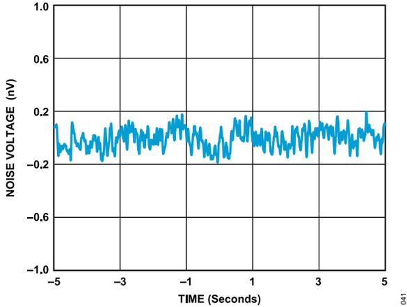
Figure 43. 0.1 Hz to 10 Hz Noise
