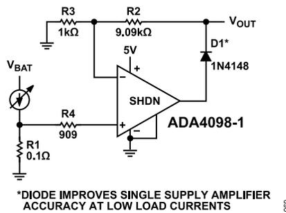
Figure 70. 1 V/A Low-Side Current Sense (ADA4098-1 6-Lead TSOT)
