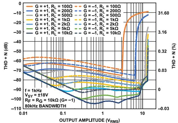
Figure 48. THD + N vs. Output Amplitude and Load
