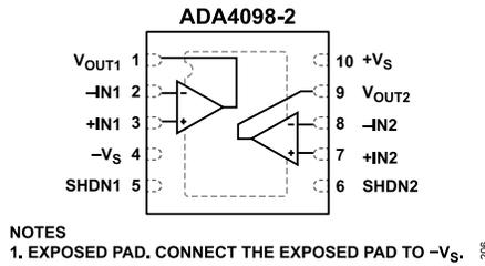
Figure 6. Pin Configuration for ADA4098-2 10-Lead LFCSP
