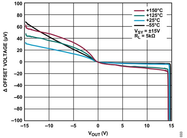
Figure 35. ΔOffset Voltage vs.  $V_{OUT}$  (5 kΩ Load)
