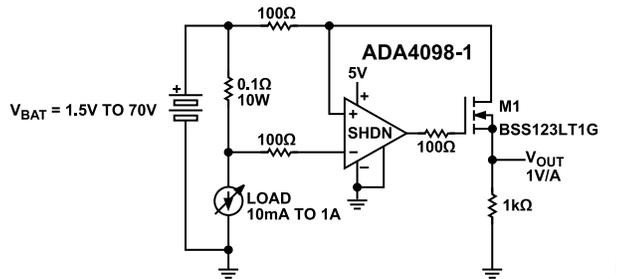
Figure 71. 1 V/A High-Side Current Sense (ADA4098-1 6-Lead TSOT)
