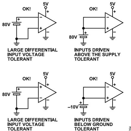
Figure 56. ADA4098-1 and ADA4098-2 Fault Tolerant Conditions
