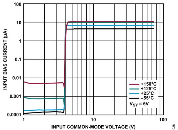
Figure 30. Input Bias Current vs. Input Common-Mode Voltage
