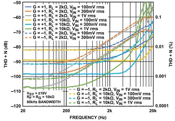
Figure 46. THD + N vs. Frequency over Load
