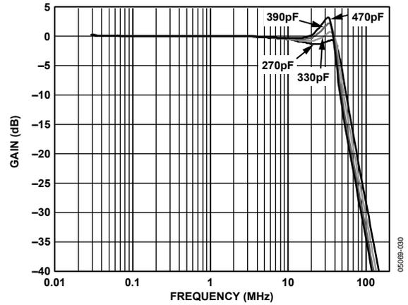
Figure 24. Capacitive Load Peaking with 2.2  $\Omega$  Series Resistor
