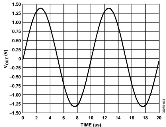
Figure 2. Output Swing,  $V_S = \pm 1.5$  V,  $R_L = 25 \Omega$
