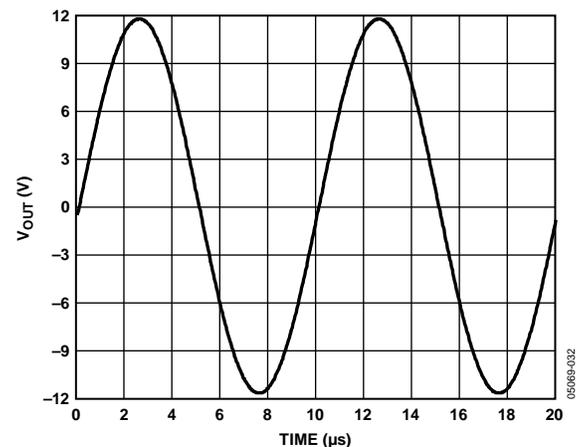
Figure 3. Output Swing,  $V_S = \pm 12$  V,  $R_L = 100 \Omega$
