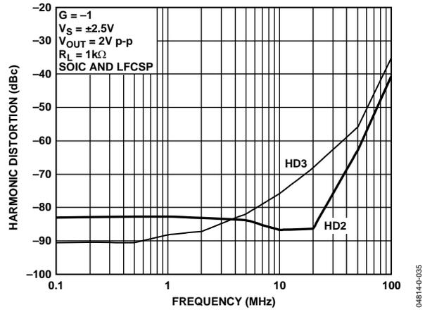
Figure 30. Harmonic Distortion vs. Frequency for Various Packages
