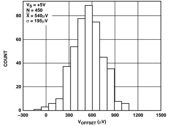
Figure 53.  $V_{OS}$  Distribution for  $V_S = +5V$
