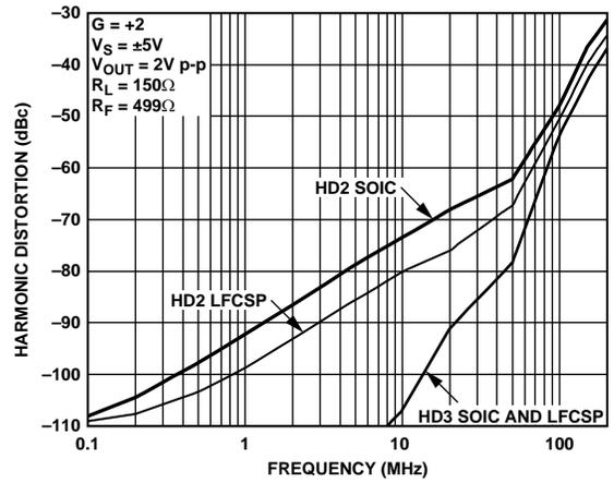
Figure 22. Harmonic Distortion vs. Frequency for Various Packages
