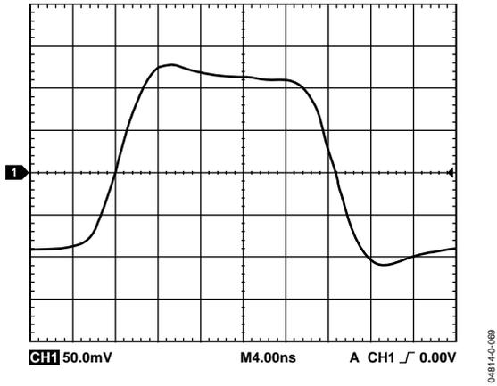
Figure 71. Small Signal Transient Response of 90 MHz LPF
