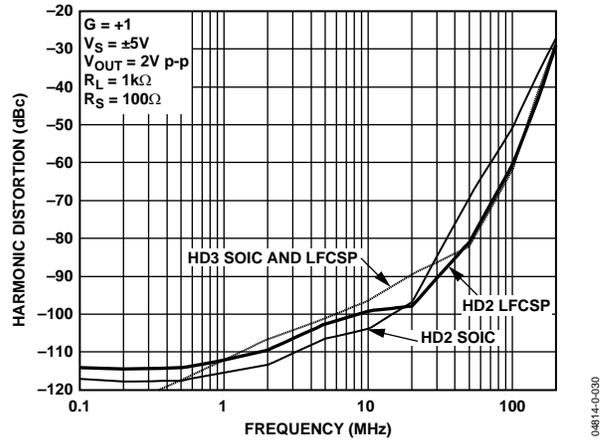
Figure 17. Harmonic Distortion vs. Frequency for Various Packages
