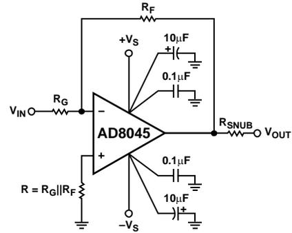
Figure 62. Inverting Configuration
