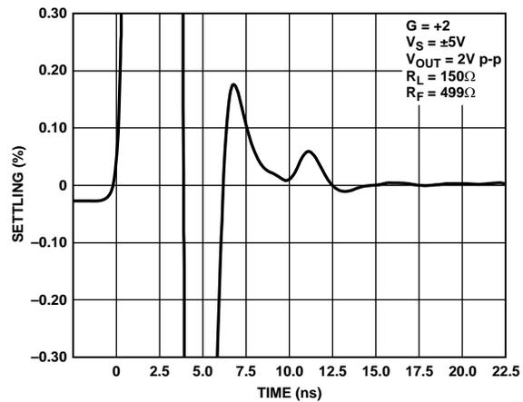
Figure 60. Short Term 0.1% Settling Time
