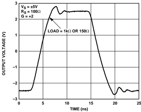
Figure 38. Large Signal Transient Response for Various Loads
