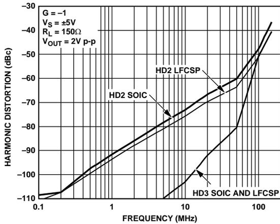
Figure 21. Harmonic Distortion vs. Frequency for Various Packages
