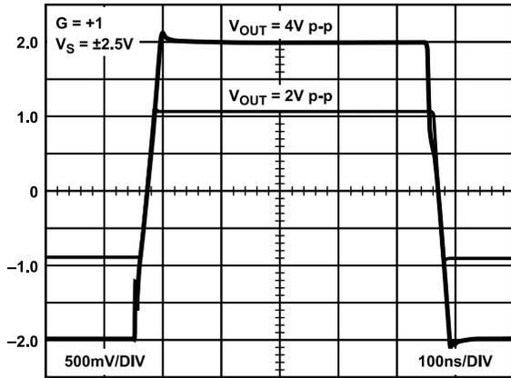
Figure 33. Large Signal Transient Response, G = +1
