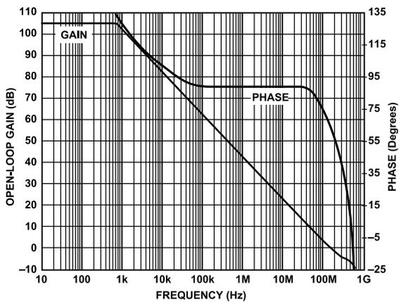
Figure 22. Open-Loop Gain and Phase vs. Frequency
