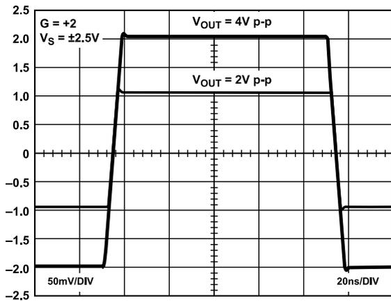
Figure 34. Large Signal Transient Response, G = +2
