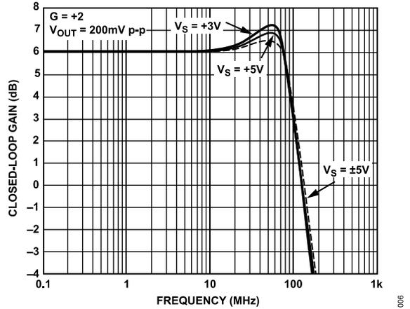
Figure 11. Small Signal Frequency Response for Various Supplies
