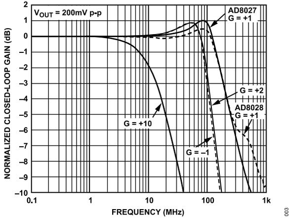
Figure 8. Small Signal Frequency Response for Various Gains
