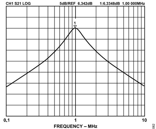
Figure 68. Band-Pass Filter Response
