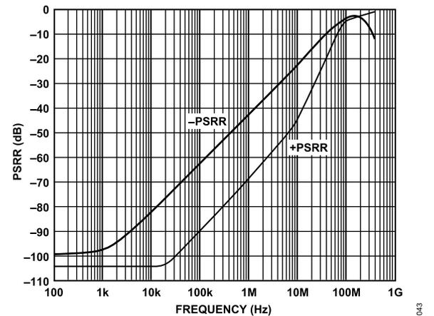
Figure 48. Power Supply Rejection Ratio (PSRR) vs. Frequency
