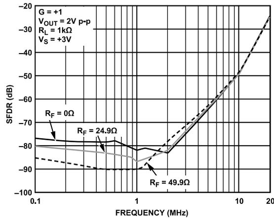
Figure 64. SFDR vs. Frequency and Various R<sub>F</sub>
