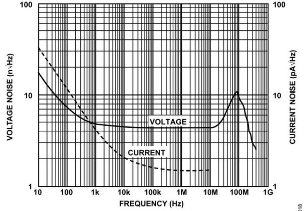
Figure 23. Voltage and Current Noise vs. Frequency
