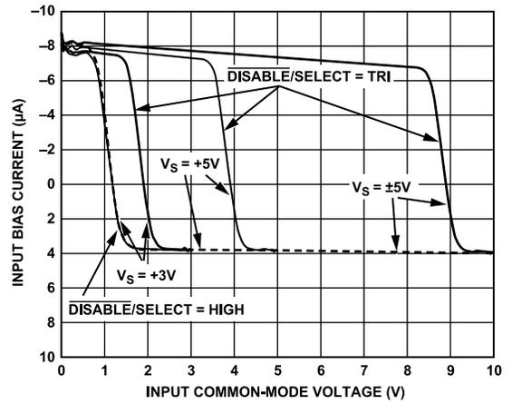
Figure 41. Input Bias Current vs. Input Common-Mode Voltage
