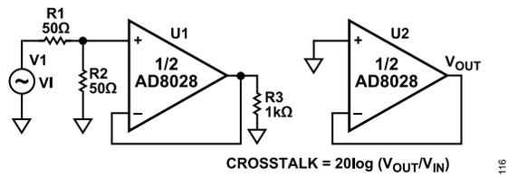
Figure 59. Crosstalk Test Circuit (see Figure 21)
