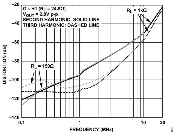
Figure 28. Harmonic Distortion vs. Frequency and Load
