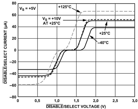
Figure 55.  $\overline{\text{DISABLE}}/\overline{\text{SELECT}}$  Current vs.  $\overline{\text{DISABLE}}/\overline{\text{SELECT}}$  Voltage and Temperature
