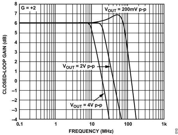
Figure 15. Frequency Response for Various Output Amplitudes
