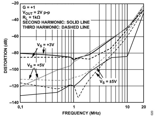
Figure 25. Harmonic Distortion vs. Frequency and Supply Voltage
