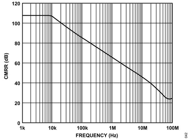
Figure 47. Common-Mode Rejection Ratio (CMRR) vs. Frequency
