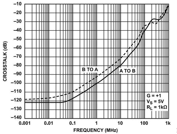
Figure 21. AD8028 Crosstalk, Output to Output (see Figure 59)
