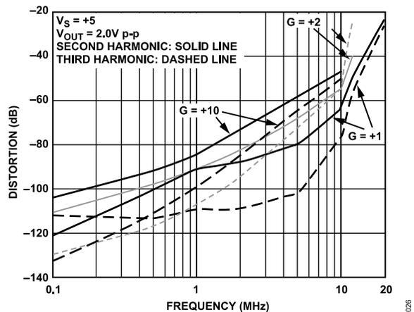
Figure 31. Harmonic Distortion vs. Frequency and Gain
