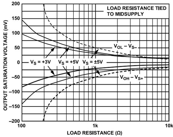
Figure 50. Output Saturation Voltage vs. Load Resistance
