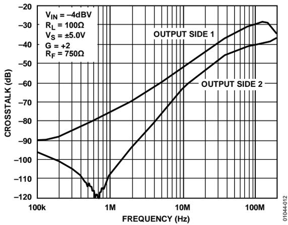
Figure 13. Crosstalk (Output to Output) vs. Frequency
