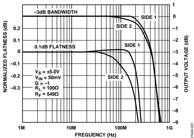
Figure 32. -3 dB Bandwidth vs. Frequency,  $G = -1$
