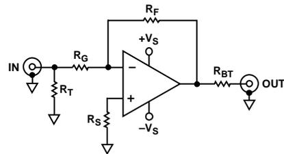
Figure 57. Inverting Configuration
