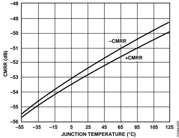
Figure 30. Common-Mode Rejection Ratio (CMRR) vs. Junction Temperature
