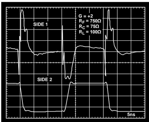
SIDE 1:  $V_{IN} = 0V$ ; 8mV/DIV RTO
