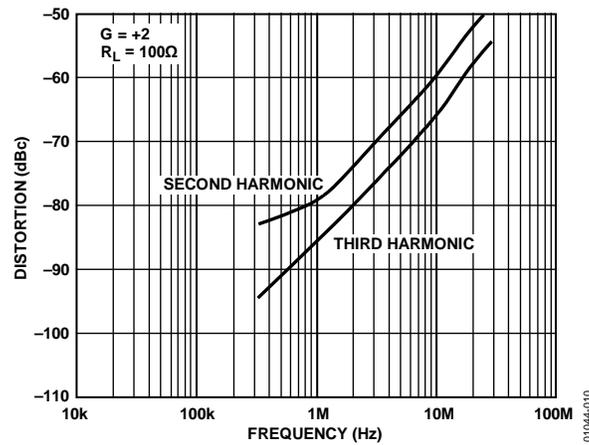
Figure 11. Distortion vs. Frequency, G = +2,  $R_L = 100 \Omega$
