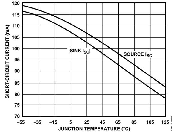
Figure 28. Short-Circuit Current vs. Junction Temperature
