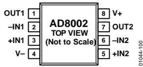
Figure 4. 8-Lead SOIC
