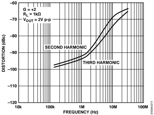
Figure 12. Distortion vs. Frequency,  $G = +2$ ,  $R_L = 1\text{ k}\Omega$
