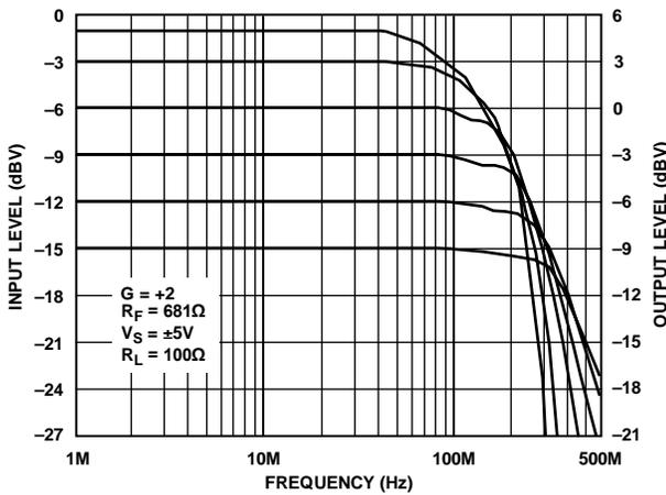
Figure 19. Large Signal Frequency Response,  $G = +2$
