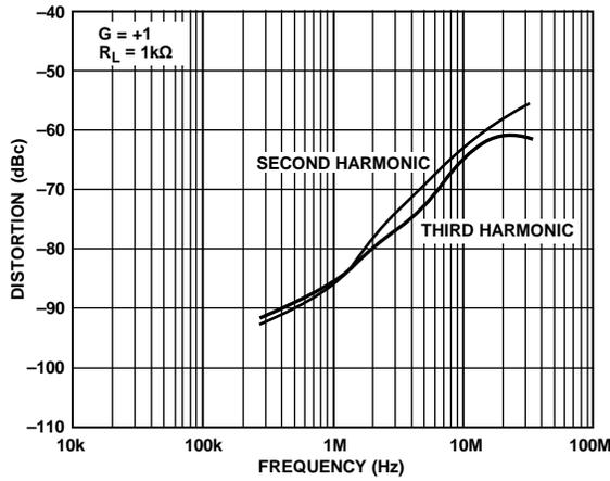
Figure 18. Distortion vs. Frequency,  $G = +1$ ,  $R_L = 1\text{ k}\Omega$
