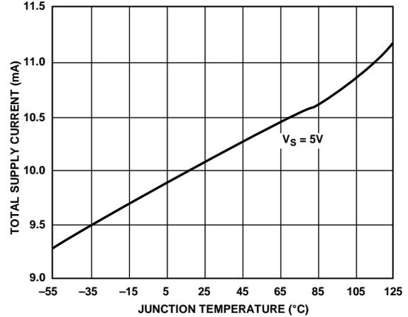
Figure 27. Total Supply Current vs. Junction Temperature
