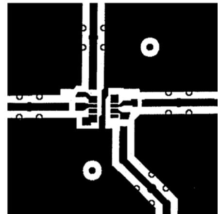
Figure 64. Inverter SOIC Board Layout (Component Layer)
