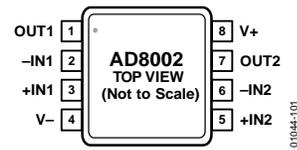
Figure 5. 8-Lead MSOP
