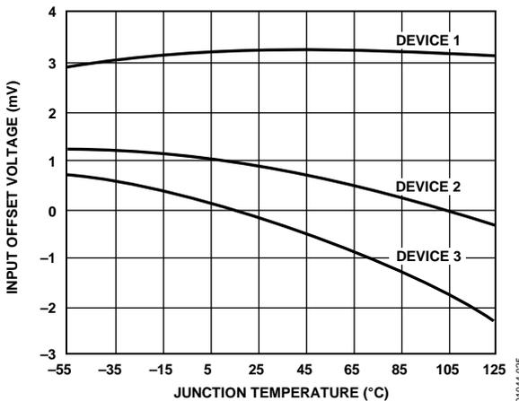
Figure 26. Input Offset Voltage vs. Junction Temperature
