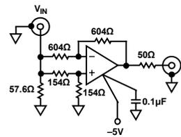
Figure 45. CMRR Test Circuit (See Figure 34)
