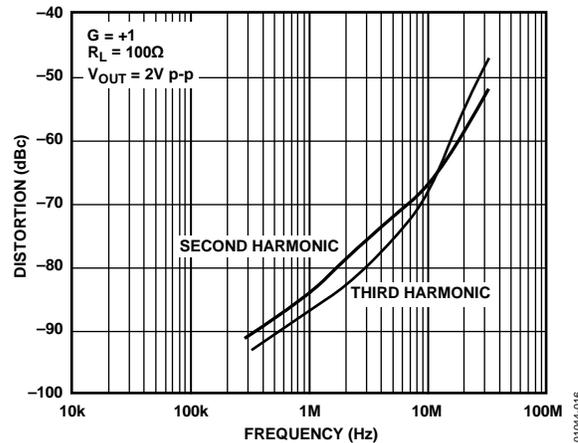
Figure 17. Distortion vs. Frequency,  $G = +1$ ,  $R_L = 100\ \Omega$
