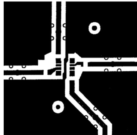
Figure 65. Noninverter SOIC Board Layout (Component Layer)
