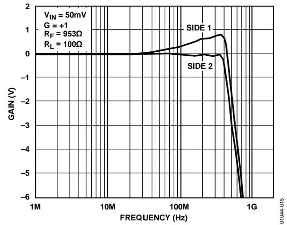
Figure 16. Gain vs. Frequency Response,  $G = +1$  (See Figure 42)
