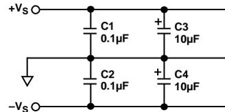
Figure 58. Supply Bypassing
