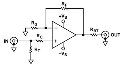
Figure 59. Noninverting Configuration
