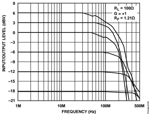
Figure 20. Large Signal Frequency Response,  $G = +1$  (See Figure 43)
