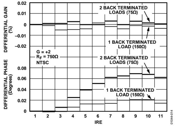
Figure 15. Differential Gain and Differential Phase (per Amplifier)
