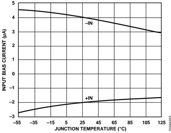
Figure 24. Input Bias Current vs. Junction Temperature
