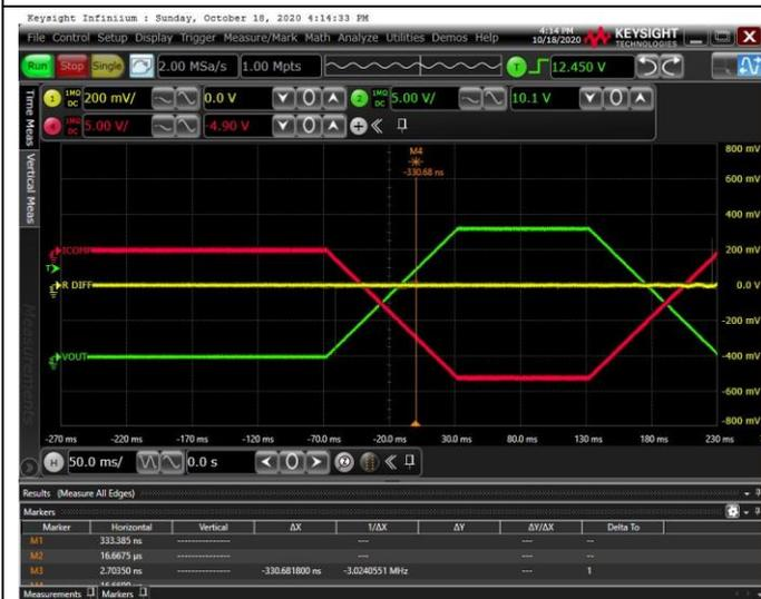
Figure 25. 100ms Power On and Off Time
