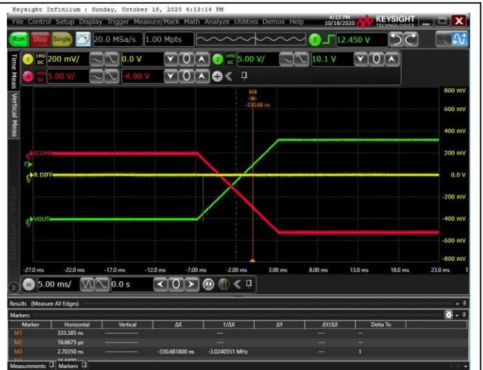
Figure 24. 10ms Power On and Off Time
