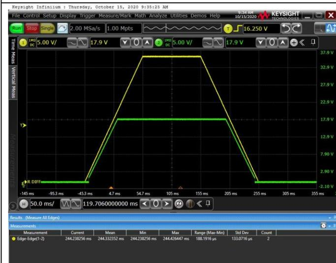
Figure 21. 100ms Power On and Off Time
