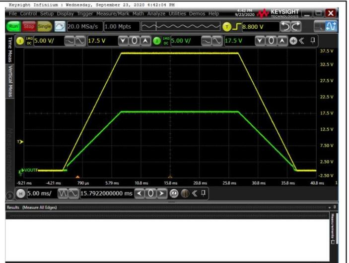
Figure 20. 10ms Power On and Off Time
