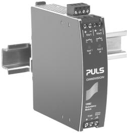
The YRM2.DIODE is a dual redundancy module, which can be used to build redundant systems. It is equipped with two input channels, which are individually decoupled by utilizing diodes.
