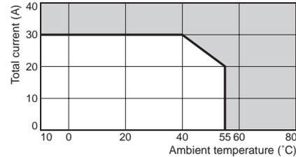
If wires with a temperature rating of 105 °C or higher are used, refer to the derating curve in *Specifications* on page 3.
