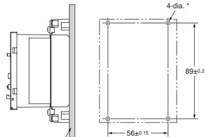
\*Diameter of pilot holes for included M4 tapping screws (guideline)
