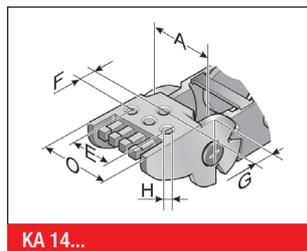
The chain bracket is a fully plastic part. The bracket is precisely adjusted to the respective chain width and only needs to be snapped in at the chain link. Please order one male and one female end bracket for each chain. The brackets should be fastened with M3 screws. The cables or conduits may be fastened with cable ties on the integrated strain relief of the chain bracket.
