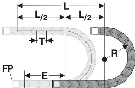
The fixed point of the cable drag chain should be connected in the middle of the travel distance. This arrangement gives the shortest connection between the fixed point and the moving consumer and thus the most efficient chain length.
