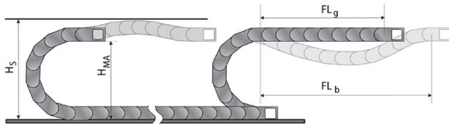
The self-supporting length is the distance between the chain bracket on the moving end and the start of the chain arch. The installation variant  $FL_g$  offers the lowest load and wear for the cable drag chain. The maximum travel parameters (speed and acceleration) can be applied for this variant.
