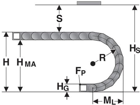
The moving end chain connection is to be screw fixed at height  $H_{MA}$  for the respective radius.
