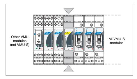
The VMU-1 has to be mounted between the group of VMU-S and all the other modules as shown in the example picture on the left.
