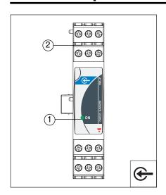
ON steady light: the module is power supplied.
