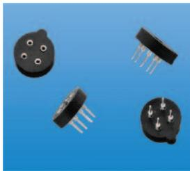
Fully molded compact construction. Speeds transistor assembly. Incorporates ultra high quality, closed entry, sleeve type contacts. Accepts .016 (.41) to .020 (.51) diameter leads or .010 (.25) x .018 (.46) rectangular transistor leads.
