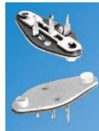
Easily assembles onto printed circuit board. Eliminates wiring. Stops on PC terminals provide sufficient spacing between socket and PC board to permit proper assembly of transistor to socket. Can be screwed down tightly to heat sink.
