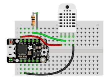
Here's an example using a Trinket MO - you can use any CircuitPython board, just check that the Data pin is pulseio - capable.
