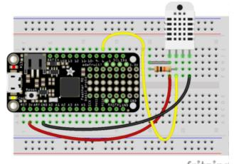
In this example we'll use a Feather M0 and DHT22 sensor connected to pin D6
